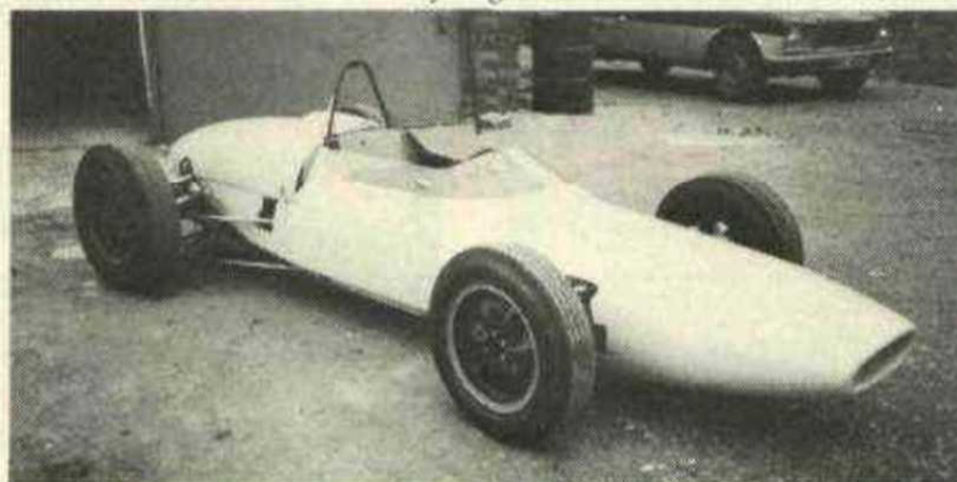
LOTUS 18/21 FORMULA ONE CAR. Thought to be Chassis Number 916. Fitted with 1½ Litre Coventry Climax engine and Colotti Type 32 gearbox. Excellent condition and ready to go.
