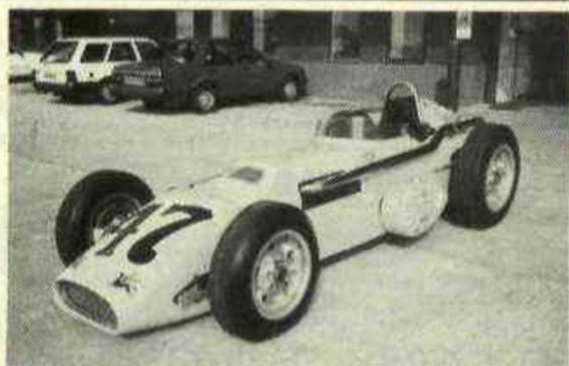
The 1959 HAYES SPECIAL INDY CAR. Offy engine. Kurtis Kraft chassis. Well known Indy car ready to see off the 250F's!
