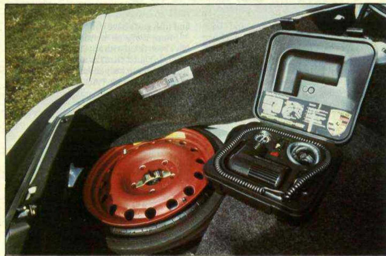
Tiny spare expands for emergencies, puffed up by neat electric compressor.
