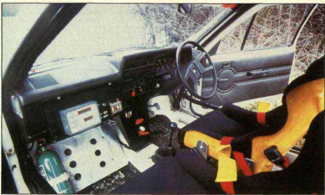
Co-driver's view is less altered than driver's; standard wheel needed for leverage.
