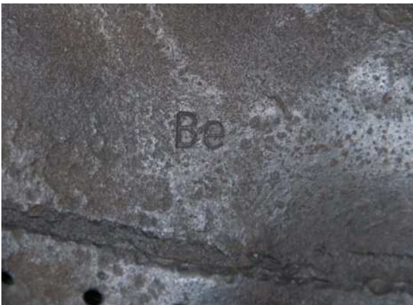
■ The "Be" marking on the combustion chamber wall.
