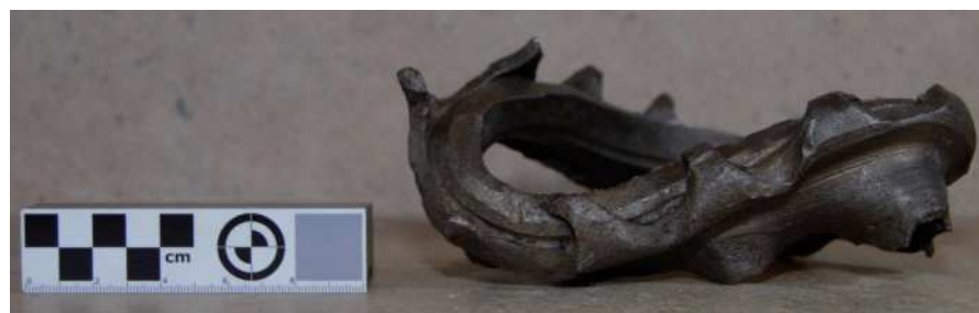
■ The conserved oxygen feed to the combustion chamber-head from the Marden V2.
