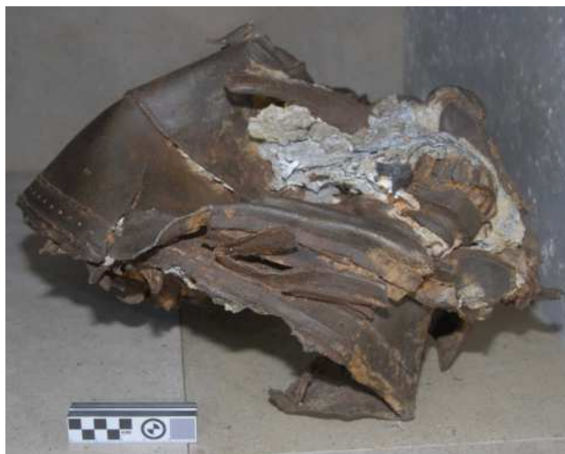
■ Left: The largest find, the conserved remains of the lower combustion chamber.
