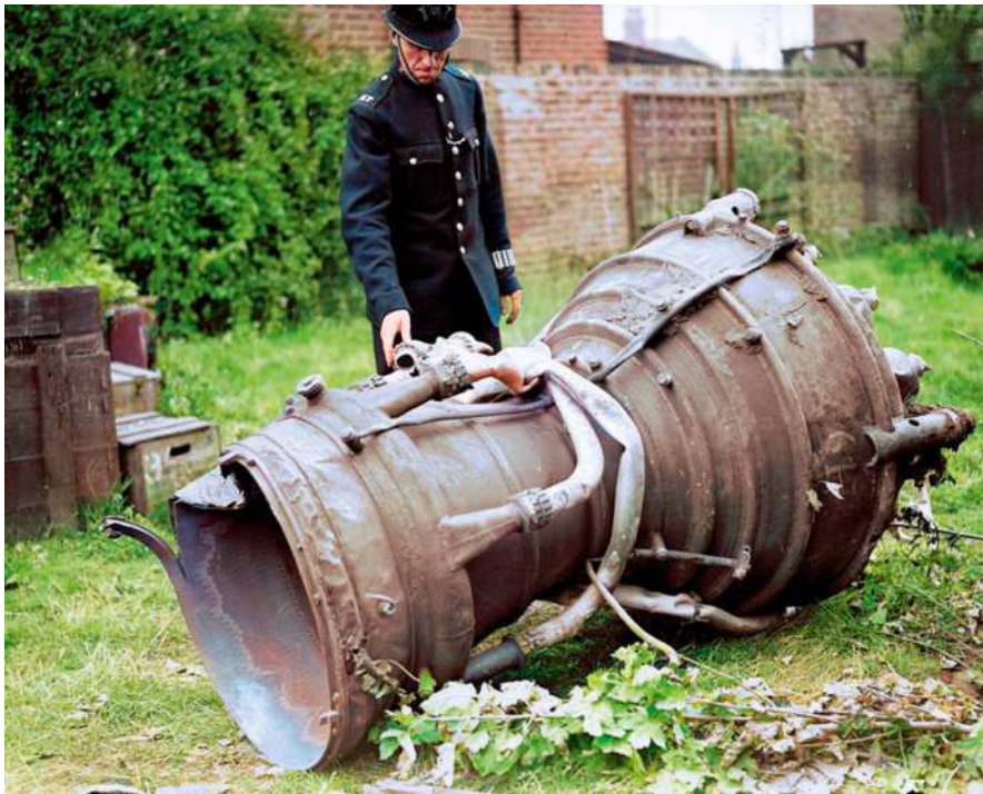
■ Sometimes, the V2 would explode or burst in mid-air prior to impact. In those instances, it was not unusual for the large combustion chamber to fall to earth relatively intact. (Photo AS. Colour by RJM)
