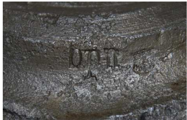
■ The Final "u" on the burner cup manufacturer's code has been accidentally applied upside-down.
