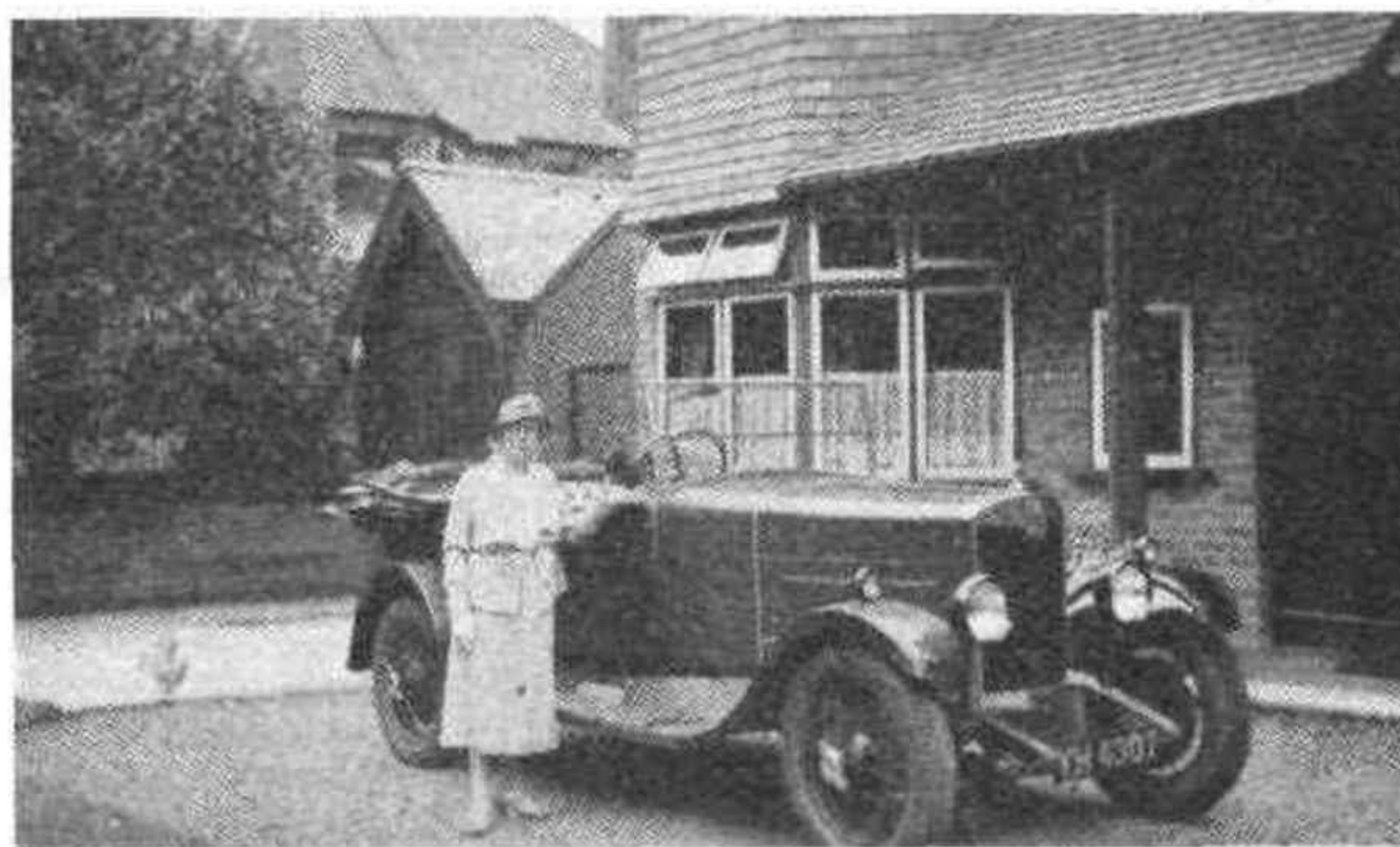
HANDSOME. —The six-cylinder twin-overhead-camshaft Lea-Francis which possessed a good chassis but suffered from an engine which was forever running big-ends and giving other trouble.
