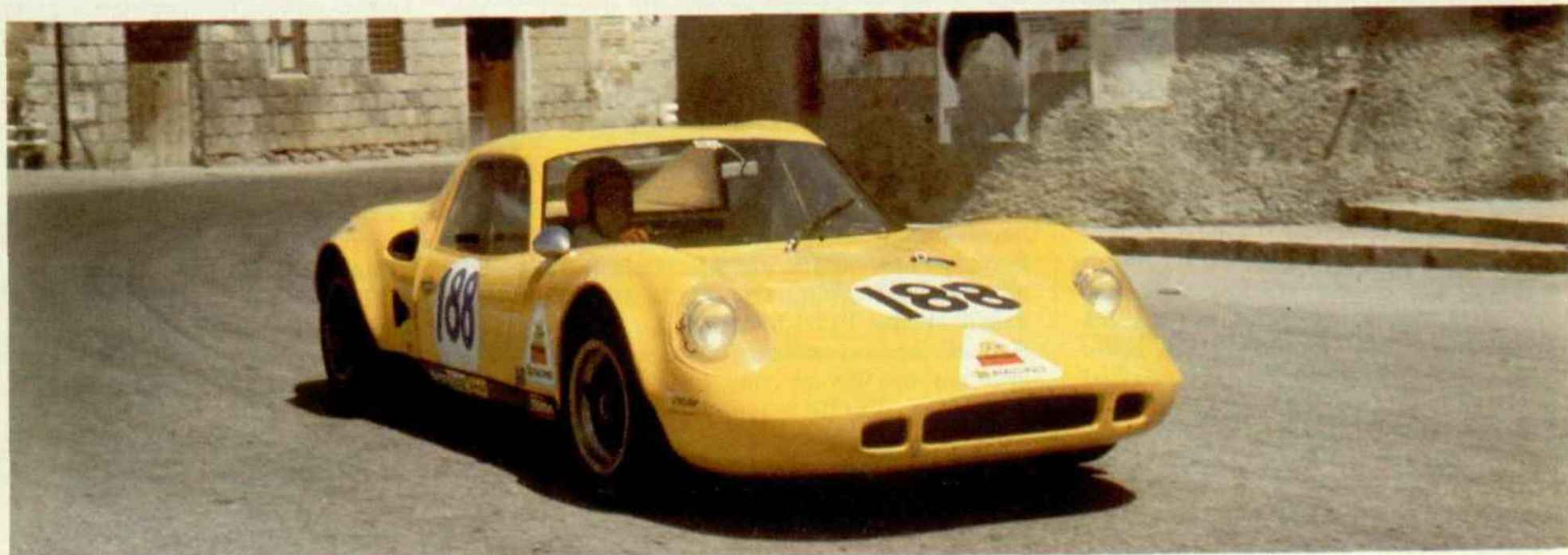
The BMW-powered B8 of Enever and Brown in the 1969 Targa Florio. Although relatively underpowered, the engine output was increased over time from 180 bhp to 230 bhp.
