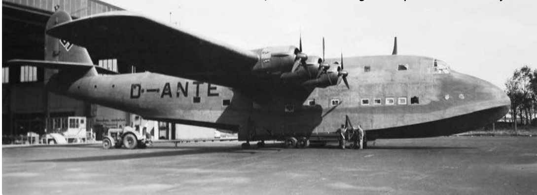
The first Blohm und Voss Bv 222 prototype, designated Bv222 V1 and given the civil registration D-ANTE, on the occasion of its roll-out at the company's factory in the Finkenwerder district of Hamburg, in August 1940. The six-engined flying-boat, originally designed to a Lufthansa specification for a transatlantic passenger aircraft, made its maiden flight on September 7 the same year.
