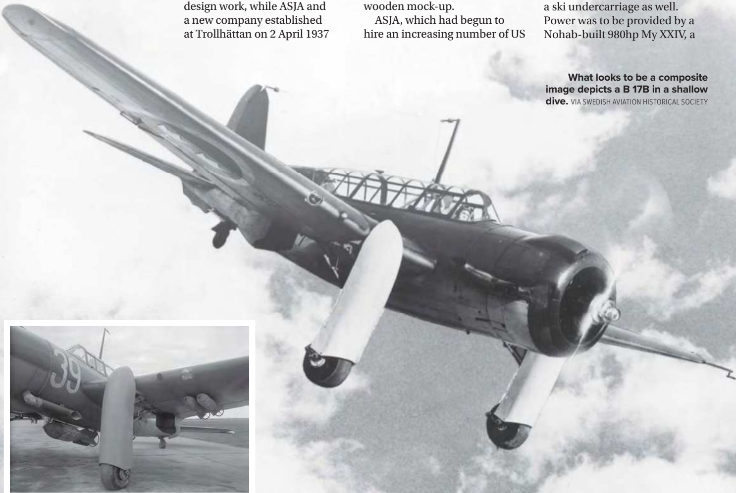
A close-up view affords detailed inspection of the undercarriage fairings that were meant to double as dive brakes, and the configuration of a bomb load.
