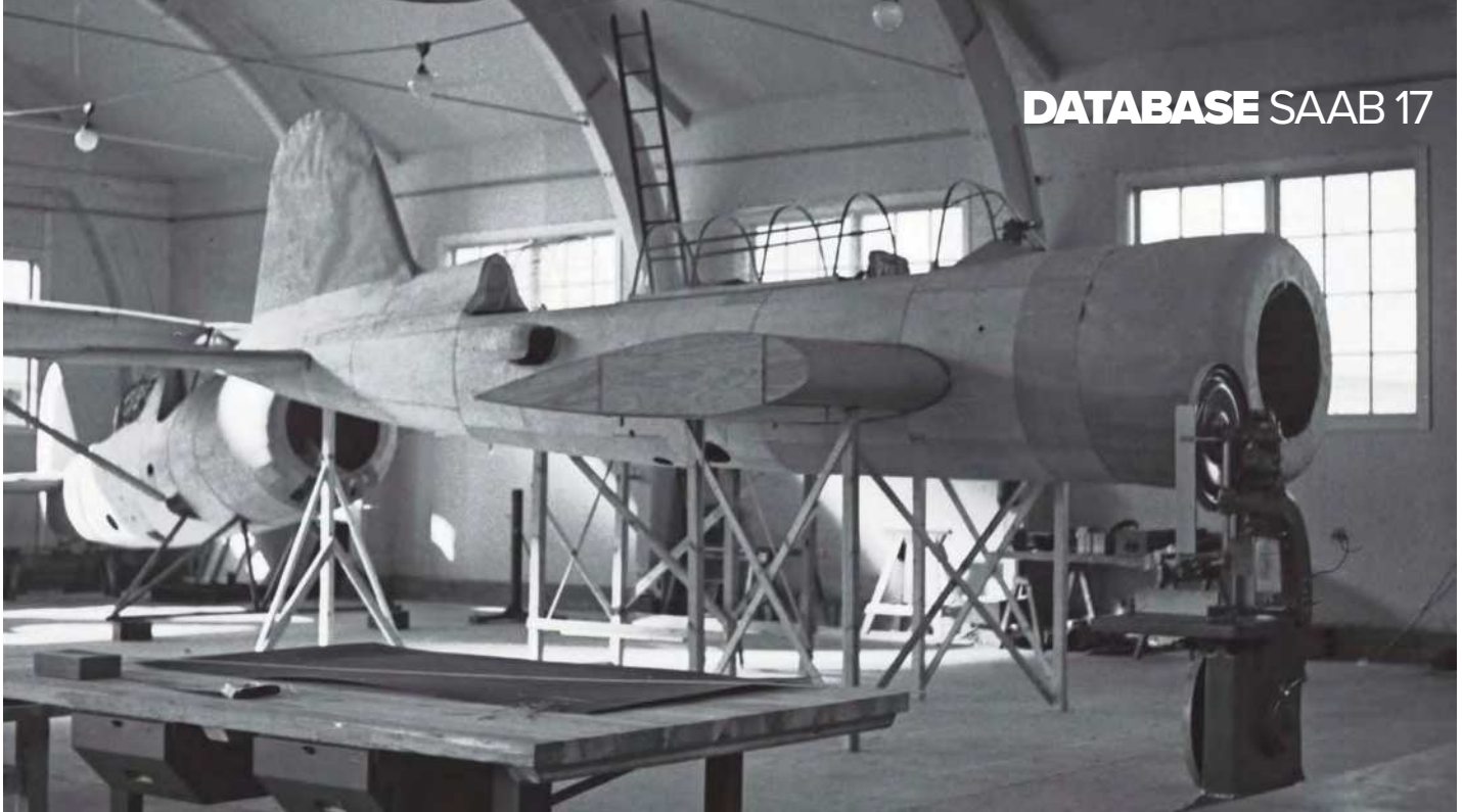
The wooden mock-up of the Saab 17, with the rejected AFF F-1 behind. VIA SWEDISH AVIATION HISTORICAL SOCIETY
