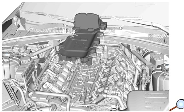
2. Remove the fuel pump insulator (1). Fuel Pump Insulator Replacement
