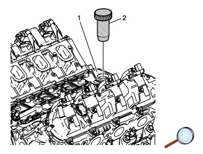
**Note:** The camshaft must be in the base circle position before the fuel pump is installed.
