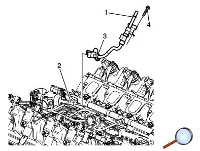
3. Remove the fuel feed pipe fastener (4) and disconnect the fuel feed pipe (1) from the fuel pump (2). <u>Metal Collar Quick Connect</u> <u>Fitting Service</u>
