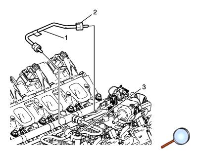
**Note:** Do NOT reuse the fuel feed intermediate pipe. If the fuel feed intermediate pipe fittings are loosened or the pipes are removed, the pipes MUST be replaced.
