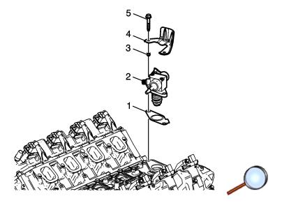
**Caution:** Alternately loosen the fuel pump bolts one turn at a time until the pump is fully disengaged from fuel pump lifter follower. Trying to remove the pump bolts without even side-to-side loosening may result in pump plunger damage
