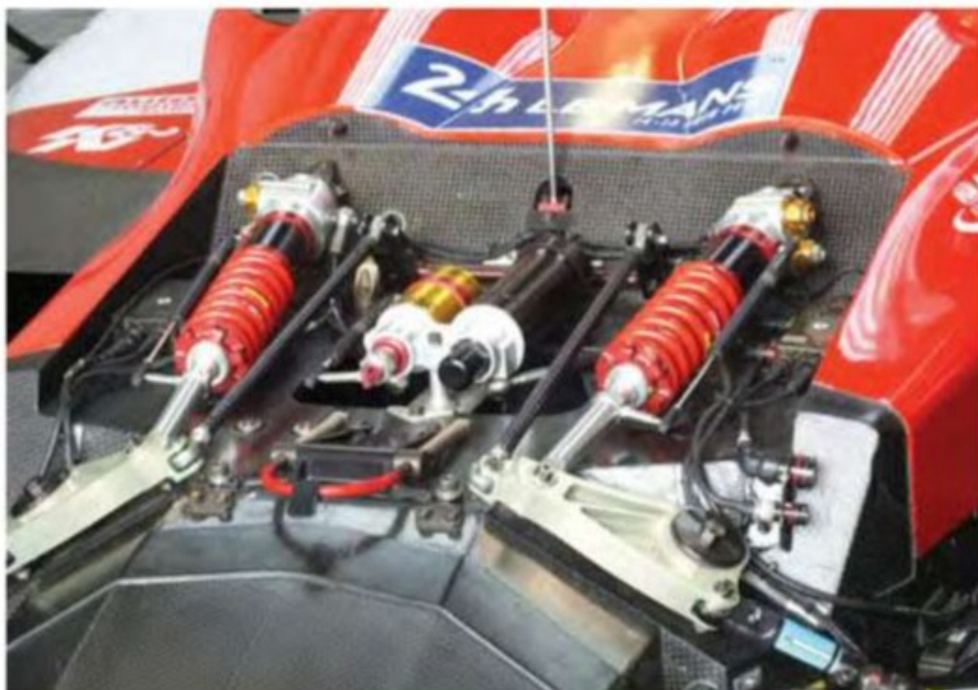
T-bar and pushrod connection setup in use on an Oreca O3R LMP2
