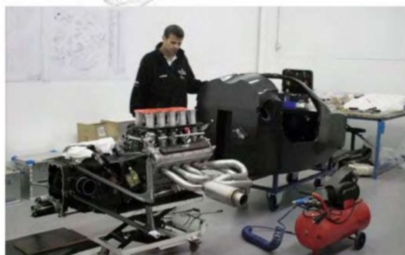
The Judd V10 meets the monocoque. The bulkhead has a cut-out for the oil tank between the upper engine mounting points
