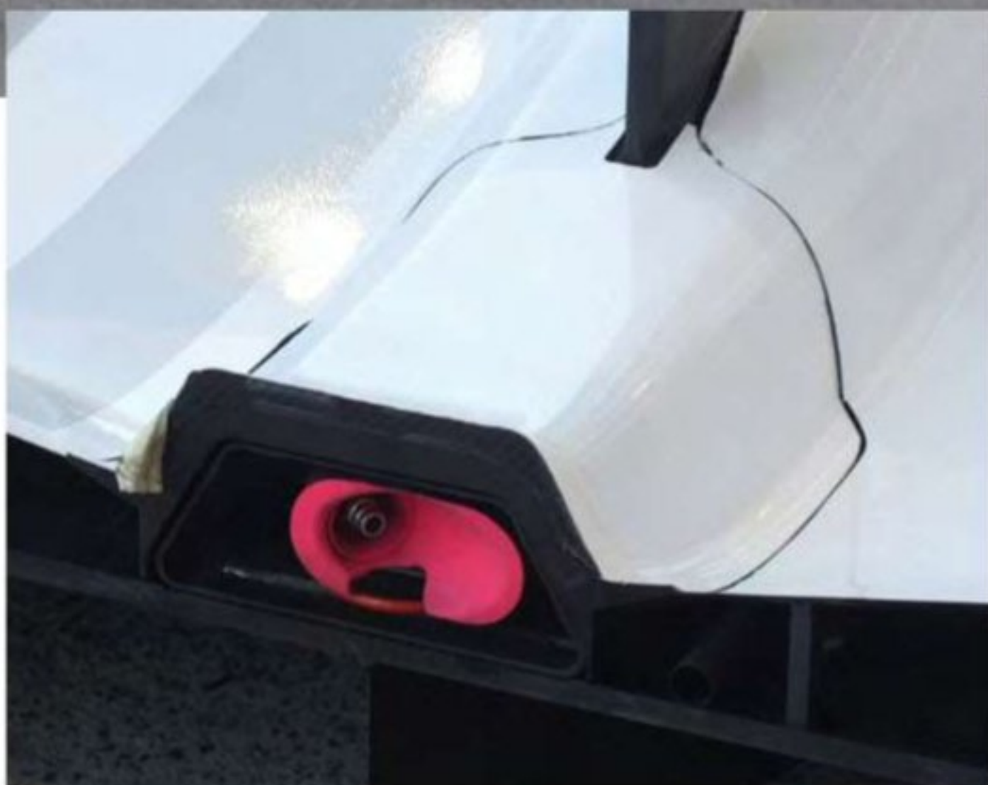
Seen at speed, the trailing edge of the rear bodywork on the Porsche 919 is deformed enough to almost contact the rear diffuser. Separation lines in the structure show where the flex is designed to occur. After protest, improvised panel supports were added to prevent movement
