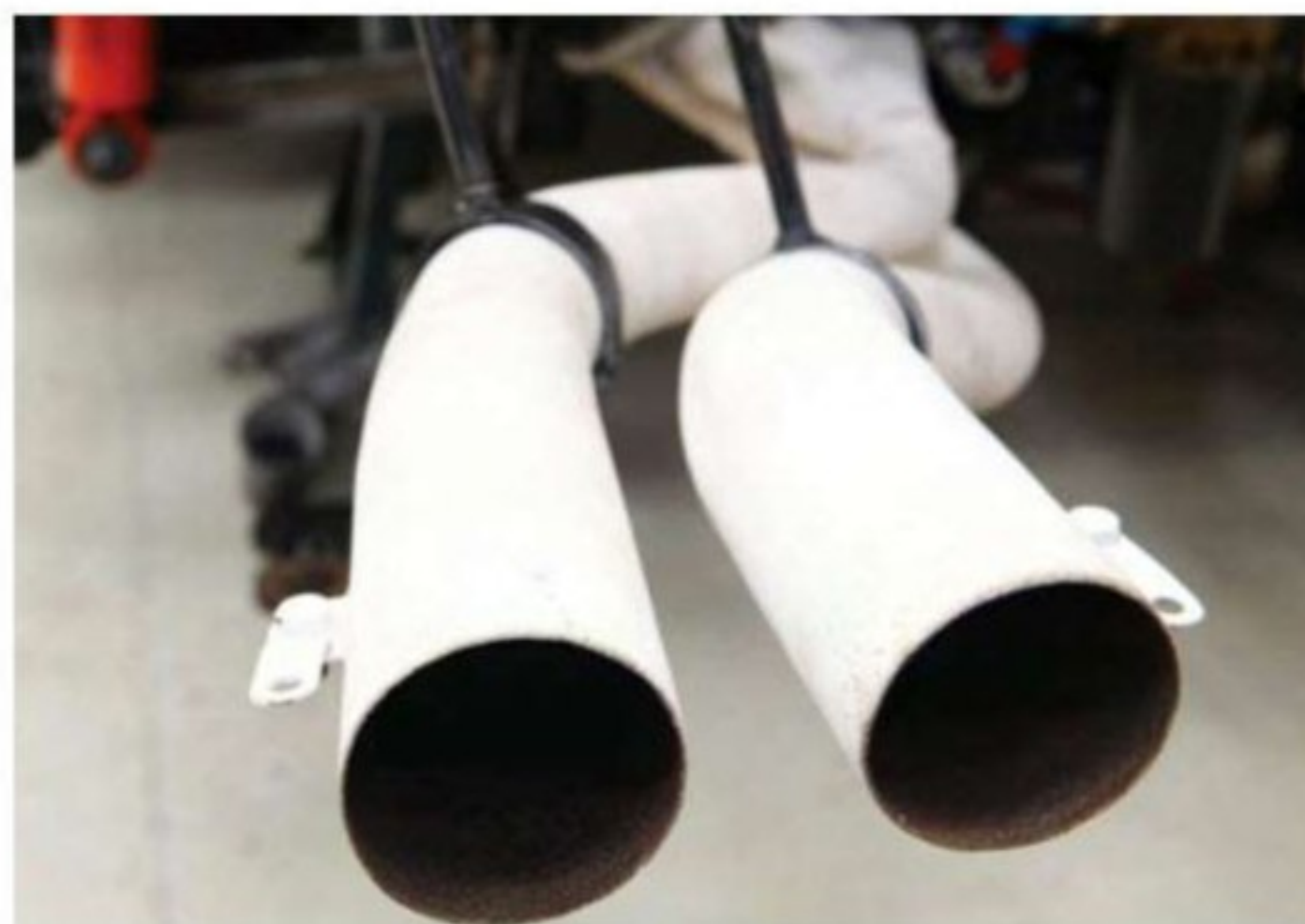
Zircotec's Performance White coating utilised on the exhaust system of historic cars
