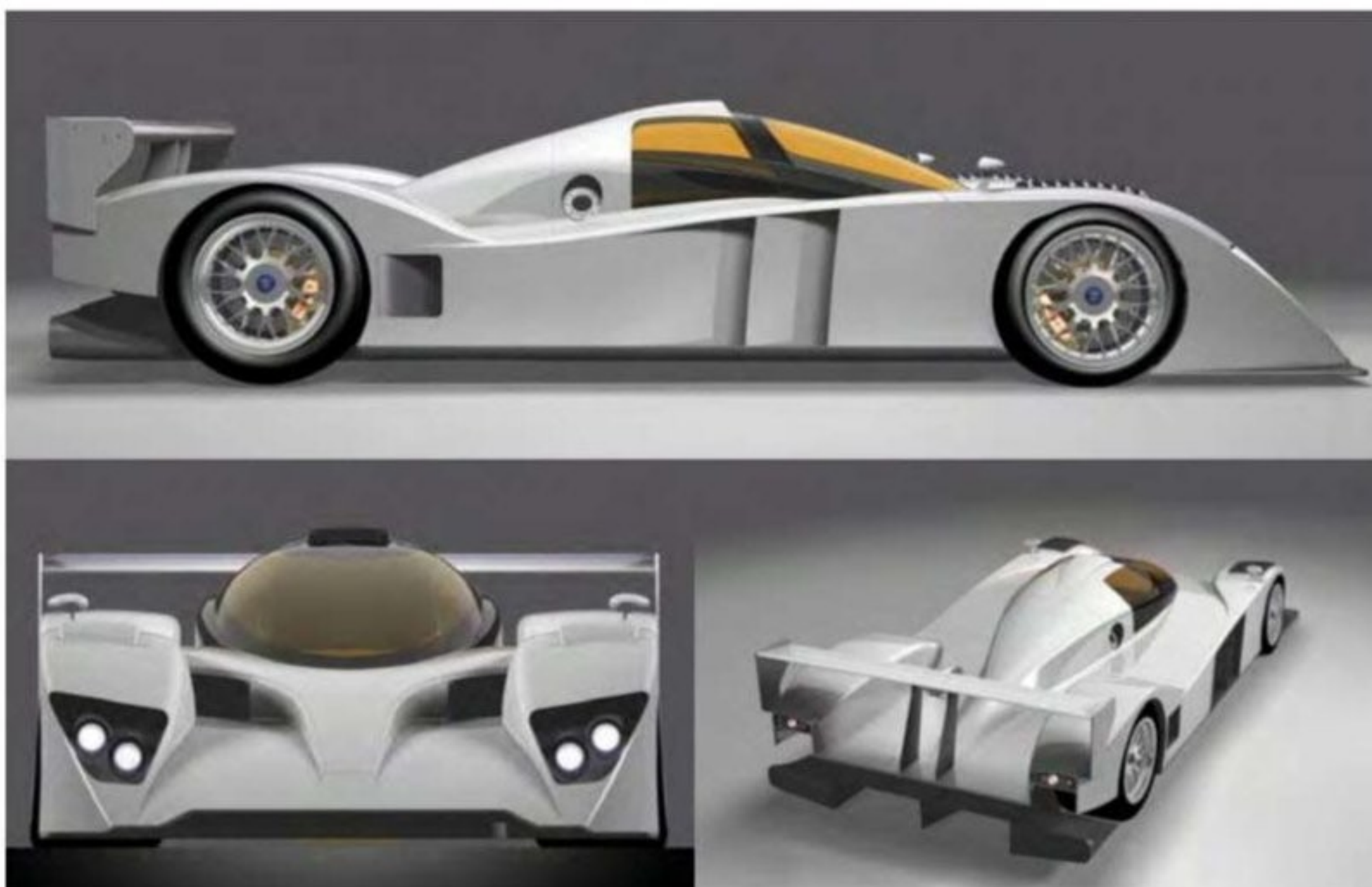
These renderings show an early version of the EE1 LMP1 car. We can see a closed front bodywork, low nose, a front splitter raised in the middle in two sections, cooling intakes besides the cockpit, a different scoop on the roof, closed sidepods with one turning vane in the diffuser exit and top mounted exhaust outlets
