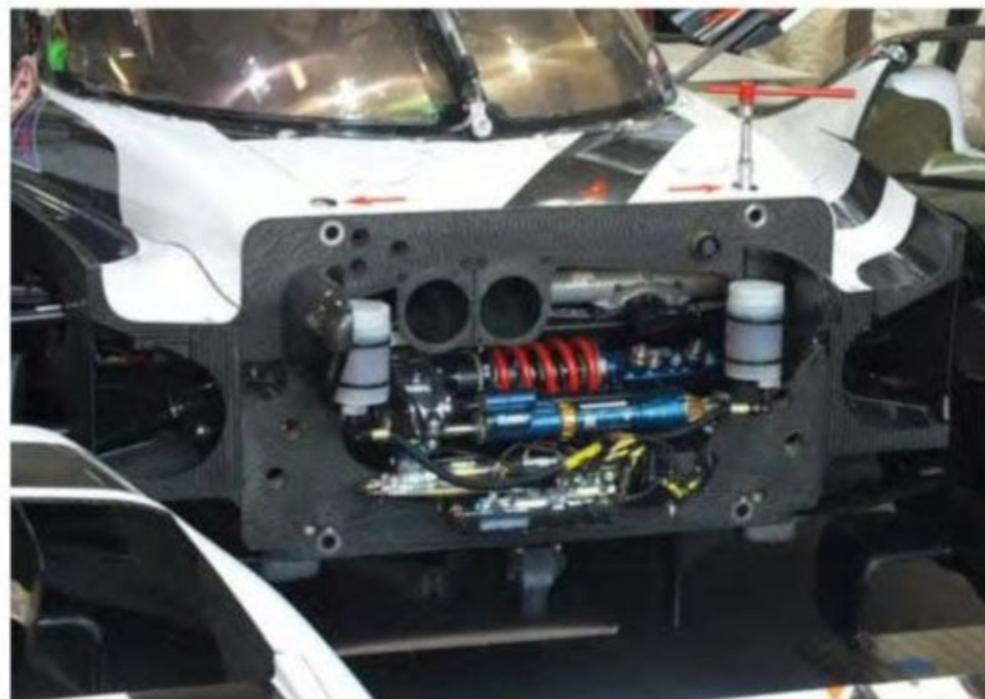
Conventional third spring systems are being superseded by advanced systems like this one on the Porsche 919. Details are as yet undisclosed
