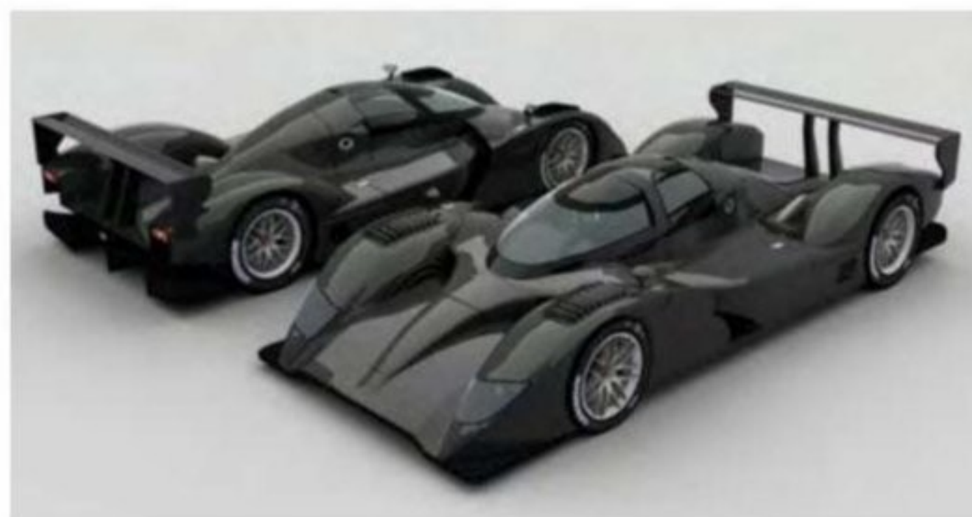
These renderings display John Travis' final version before the Peugeot 908 appeared. We see still a strong resemblance to the version in the pictures above but the front fenders are now open at the rear and the sidepods are scalloped at the underside of the leading edge to create a larger front diffuser exit area. Note also the small NACA-duct in the engine cover. This was later changed to serve the engine with more air
