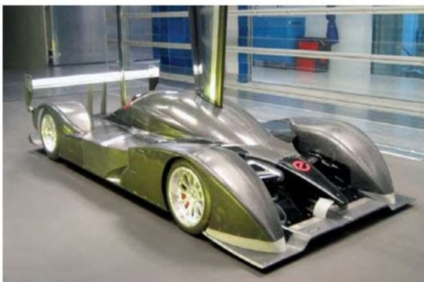
The 40 per cent wind tunnel model in the Aerolab wind tunnel. The rear fender is not connected to the diffuser, unlike the carbon render above
