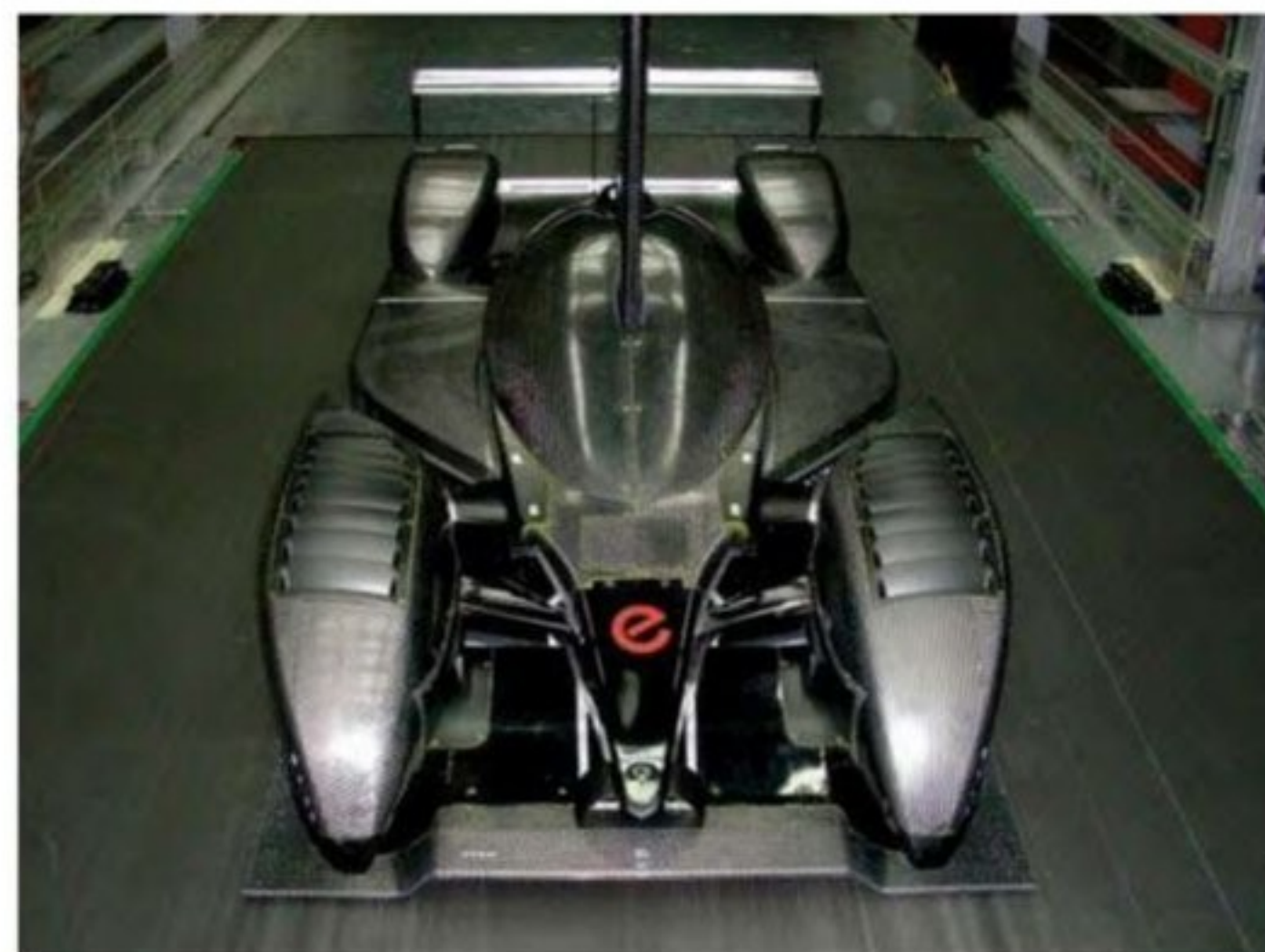
This wind tunnel model shows louvred panels on the front wheel fairings. But more interesting are the different valance panels. We see the same wheel fairings as in the model above but then we have a small valance panel above the wheel fairings and a second pair connected to the sidepods directly above the cooling intake. This arrangement shows similarities to the Peugeot 908 version
