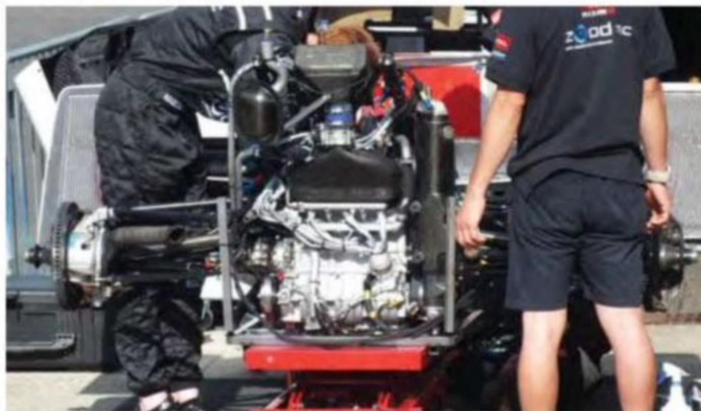
Rarely seen view of the engine in situ with rear suspension and radiators
