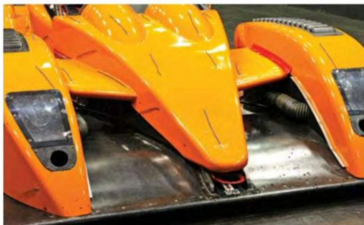
Picture 3: Removing the nose infills had a significant effect
