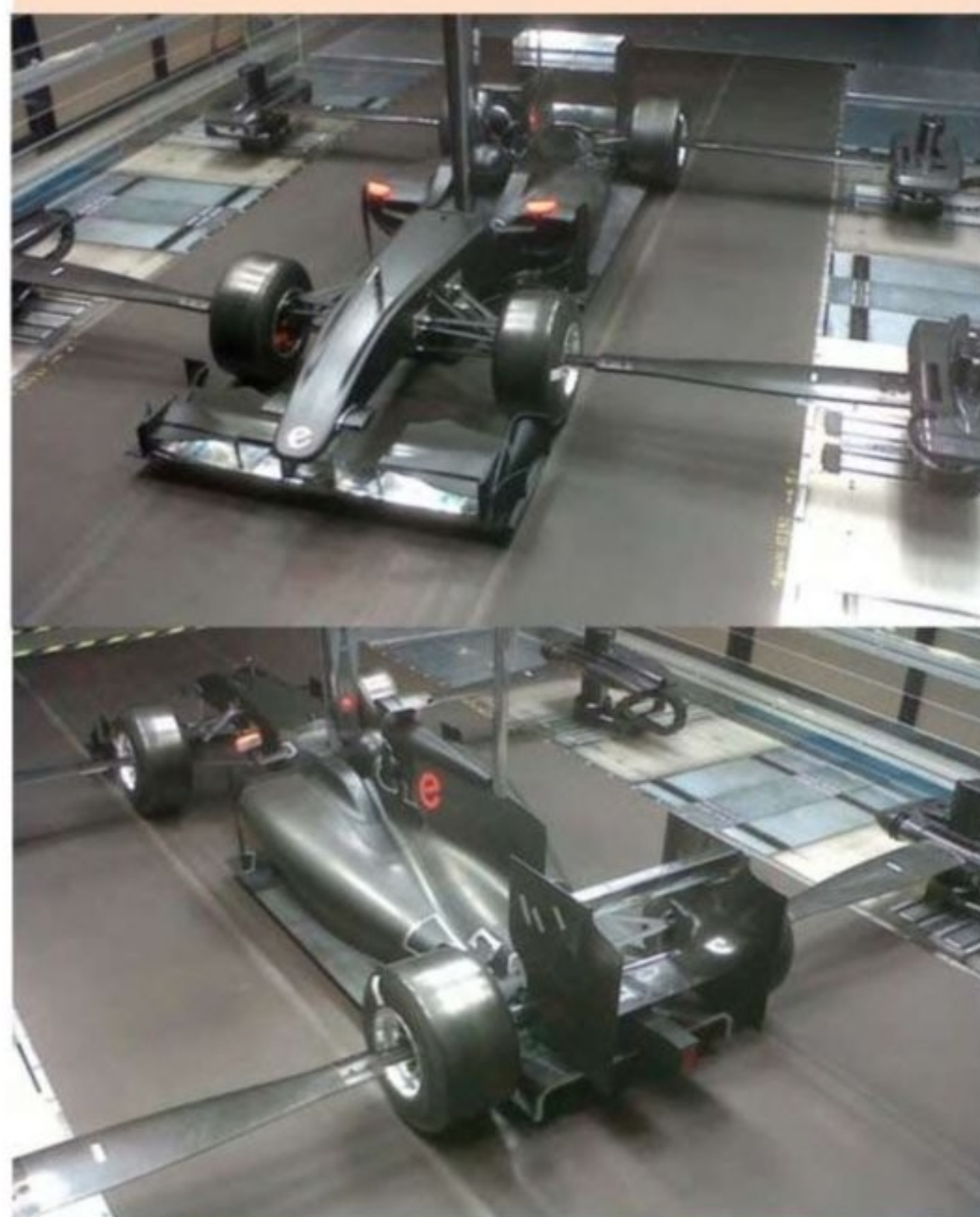
The pictures above show the stillborn 2011 Epsilon Euskadi F1 car in the wind tunnel. Compared to contemporary Virgin and HRT cars, this represents a much more advanced design
