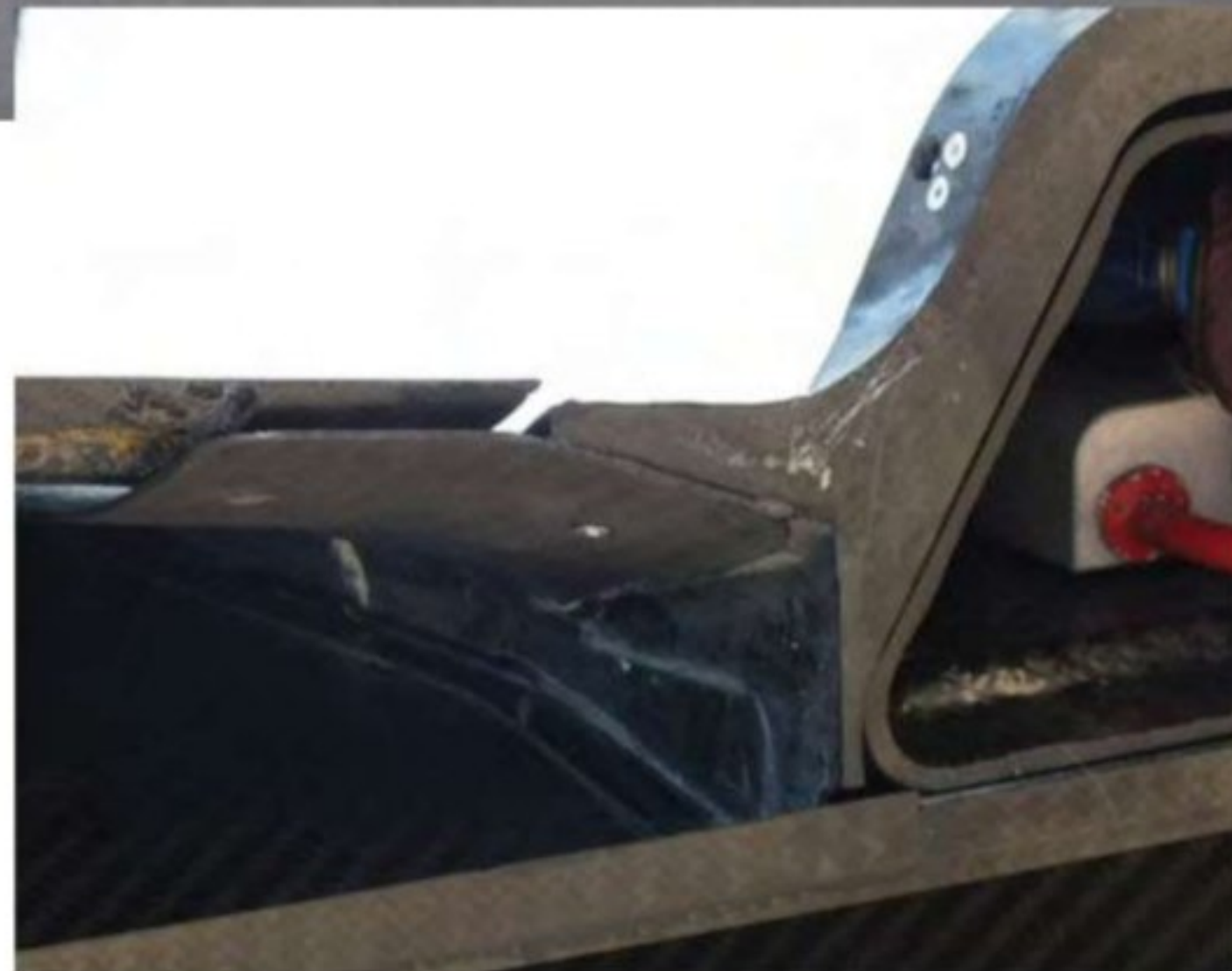
Seen at speed, the trailing edge of the rear bodywork on the Porsche 919 is deformed enough to almost contact the rear diffuser. Separation lines in the structure show where the flex is designed to occur. After protest, improvised panel supports were added to prevent movement
