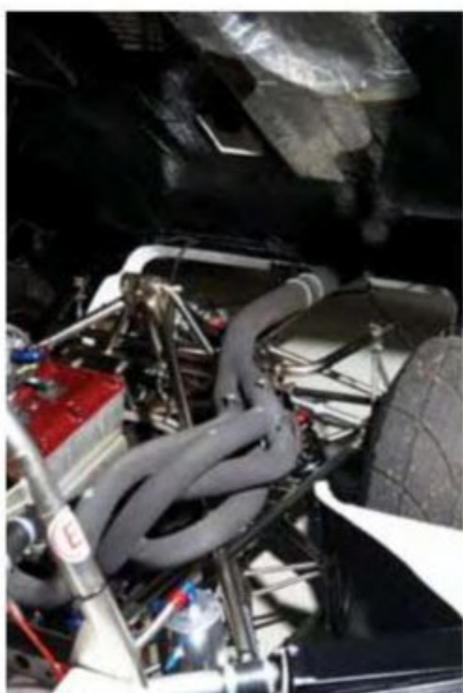
Zircotec's Performance White coating utilised on the exhaust system of historic cars
