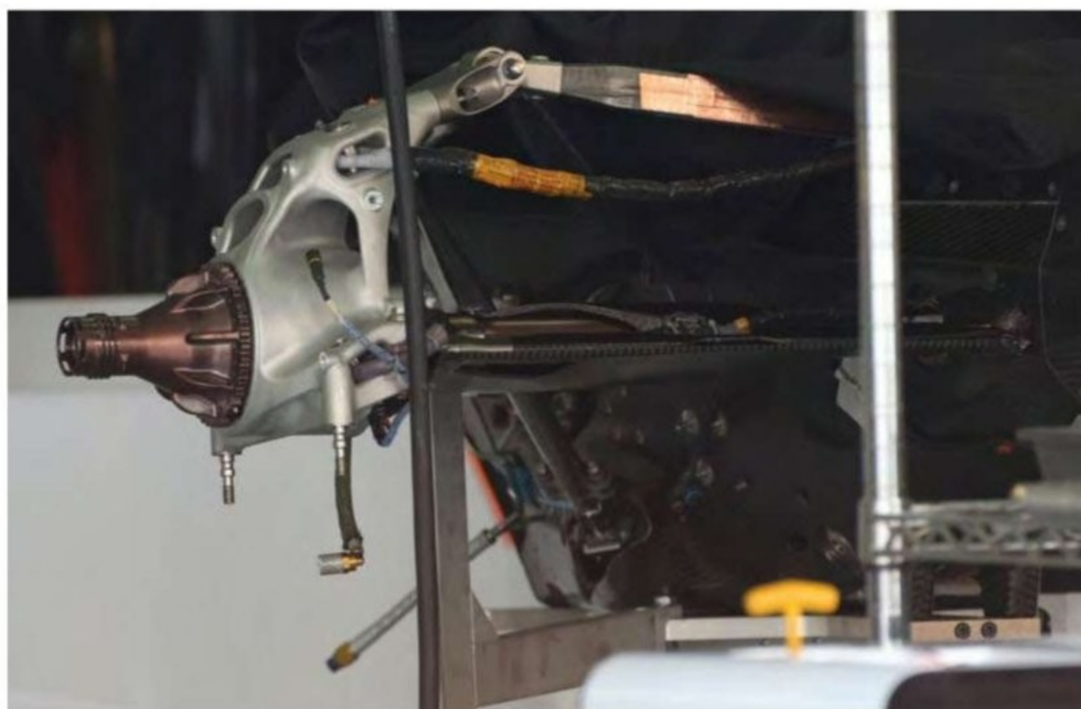
The intricate organic design of the rear suspension uprights has drawn a lot of interest
