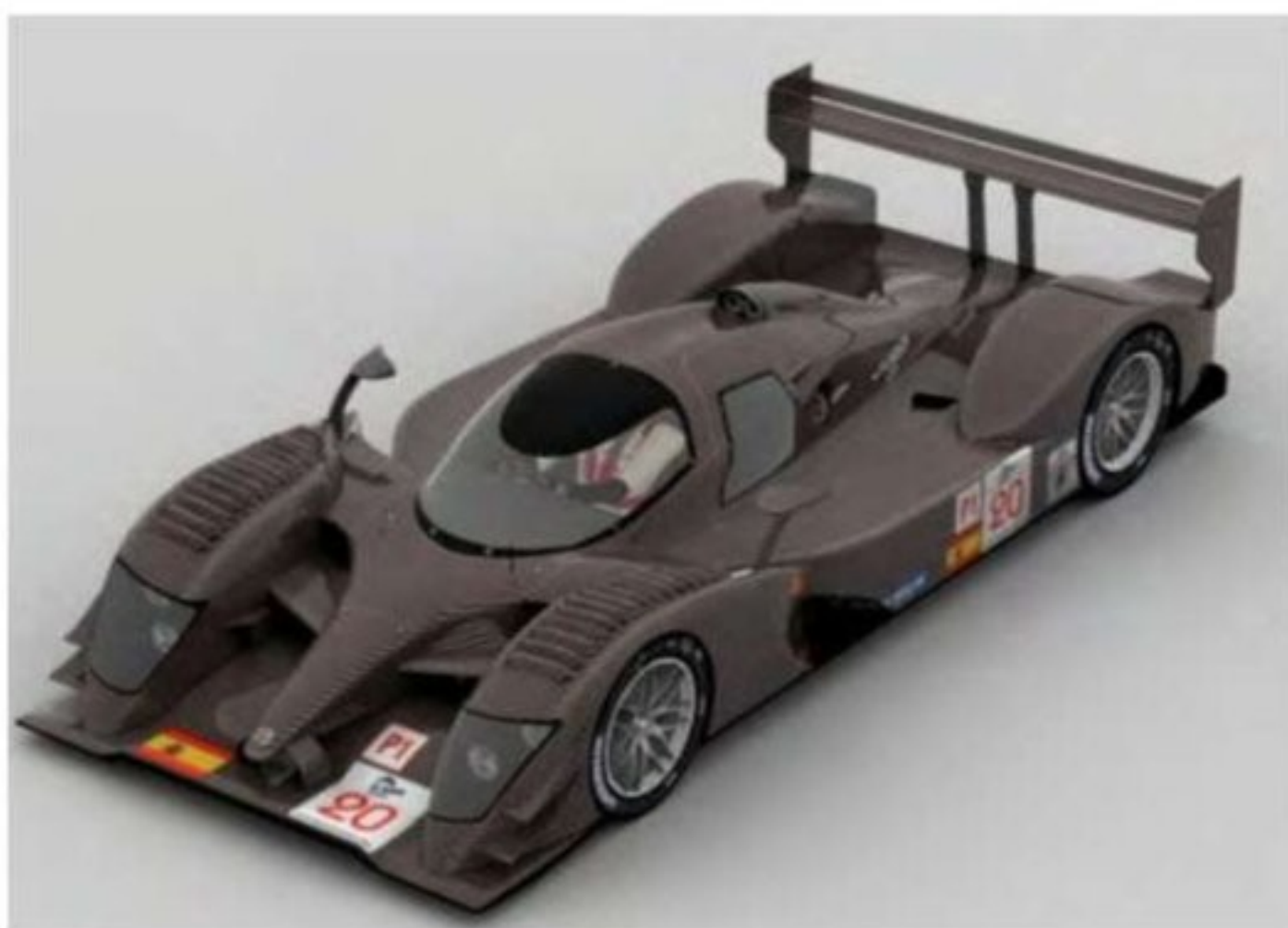
This rendering shows the final EE1 layout with a small high nose, open front bodywork with wheel fairings with the air directed to the cooling intakes via the suspension, lower scalloped sidepods and a new scoop on the engine cover
