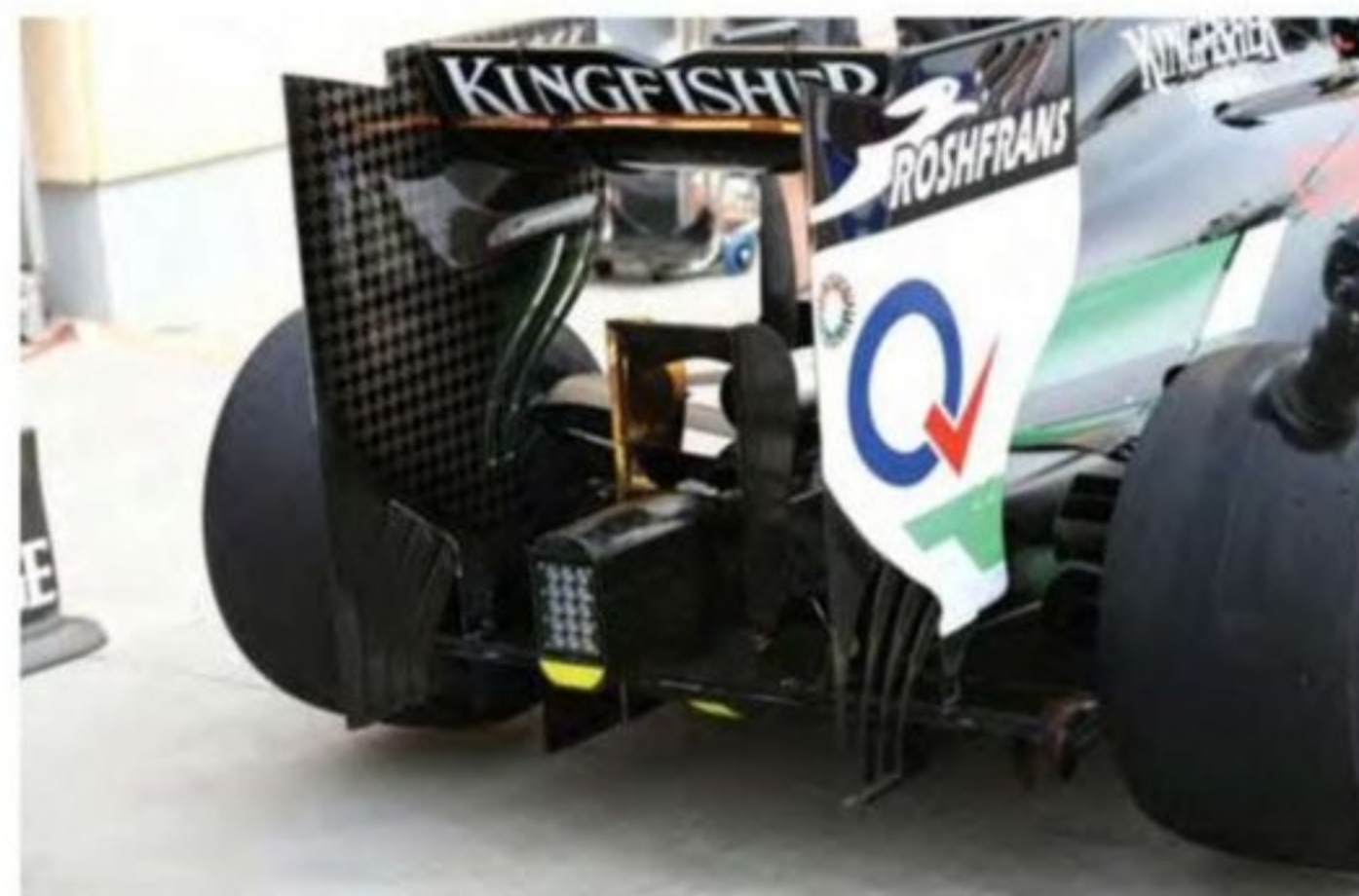
The aero-assisting Coanda exhaust system is outlawed for 2014, with all cars now restricted to a single central tailpipe
