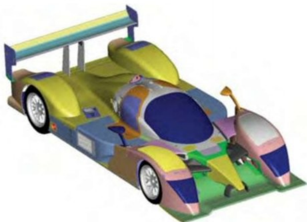
Colour coded view clarifies the individual bodywork panels of the refined high nose EE1. Note intake scoop replacing original NACA duct
