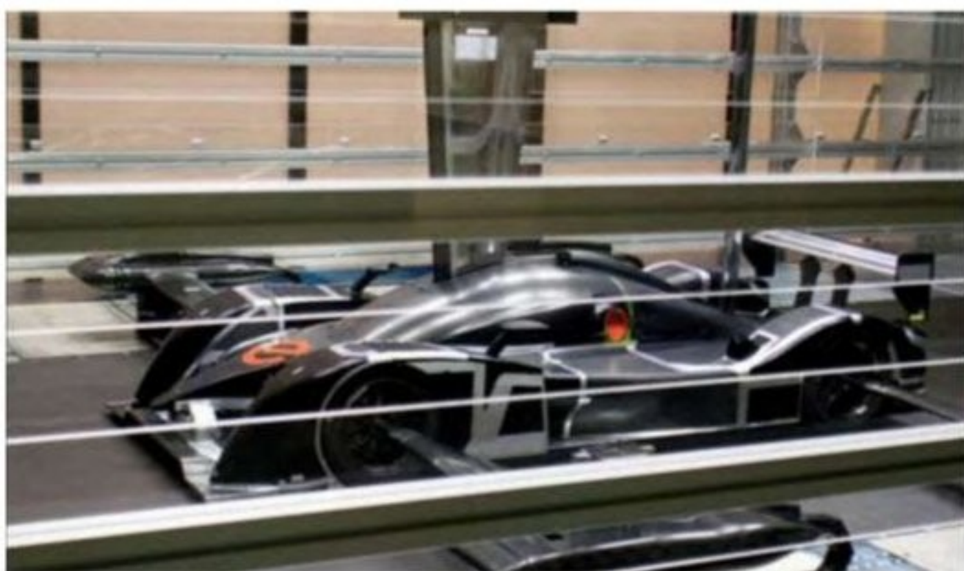
The 40 per cent wind tunnel model of the EE2 in the Aerolab tunnel. Obvious changes are the new rear brake scoops on the rear fender and the much more scalloped sidepods
