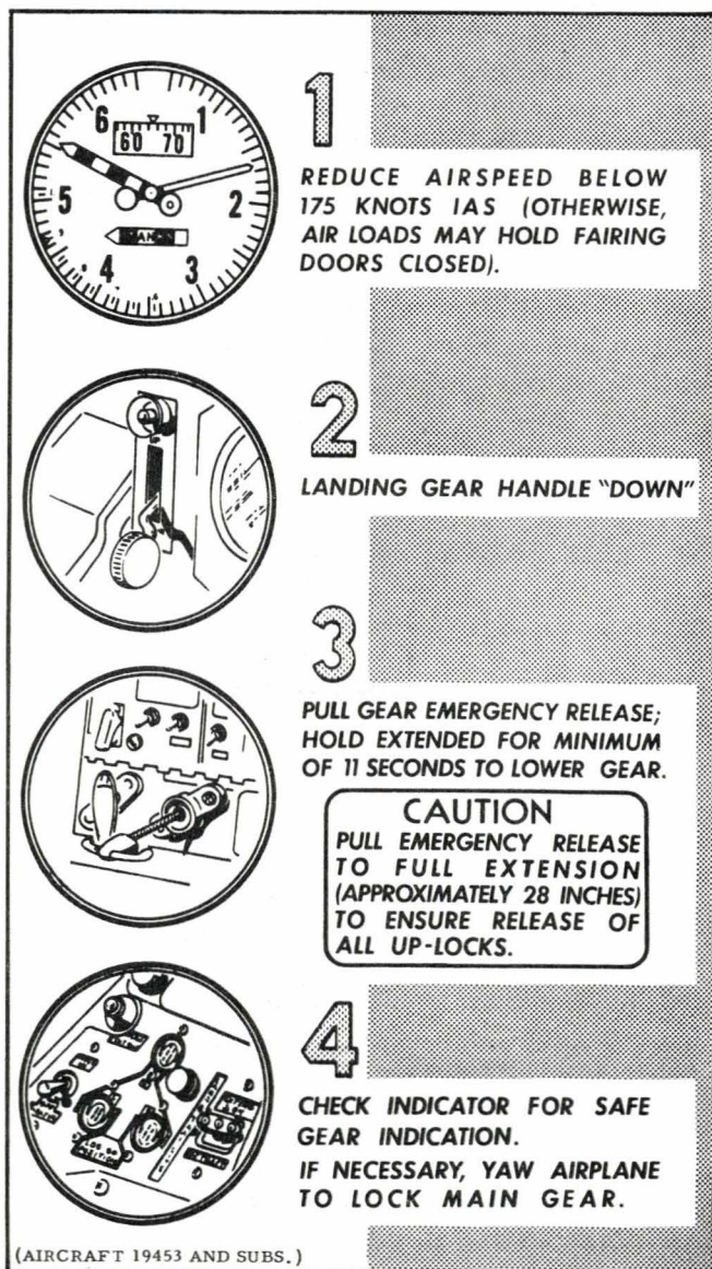
Figure 3-2 Landing Gear Emergency Extension (Aircraft 19453 and Subsequent)
