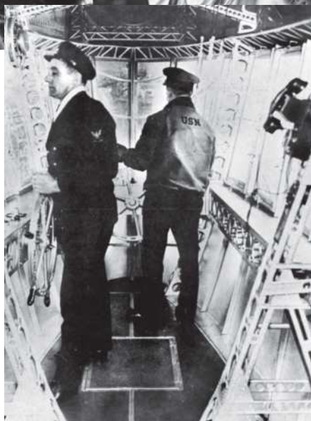
ABOVE: This view aboard the airship USS Macon was taken in the auxiliary control station in the lower vertical fin sometime between 1933 and 1935. TOP: U.S. Navy sailors work amid the steel superstructure of the airship USS Macon (ZRS-5) during the 1930s. Macon was constructed at the Goodyear Airdock in Springfield Township, Ohio, by the Goodyear-Zeppelin Corporation.
