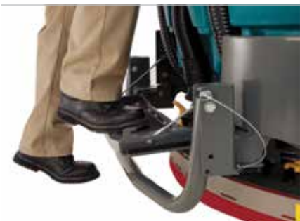
Recovery Tank Access Step
