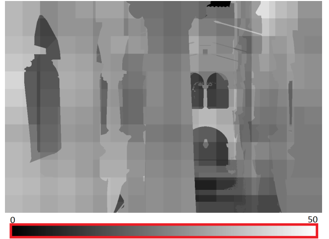
Figure 4: The color grading describes the number of light calculations per fragment. Black is 0 lights and white is 50 lights.
