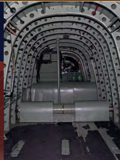
Centre left The bomb bay doors will also have to be removed.
