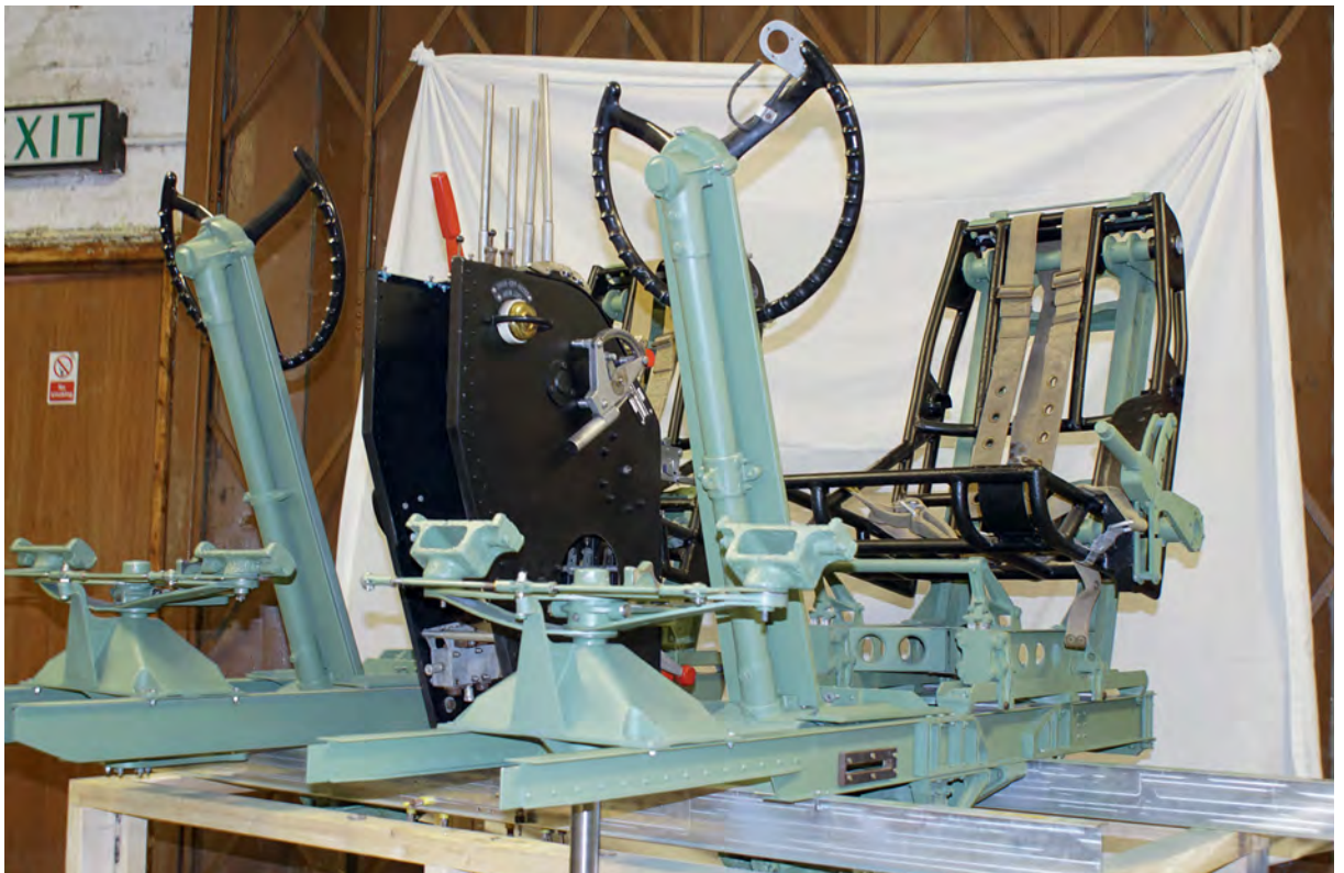
Right Pilots' seats, throttle box and control columns, destined to be the centrepiece of the project's forward fuselage.
