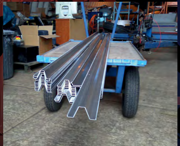
Above Part of the stock of stringer sections manufactured for the project.
