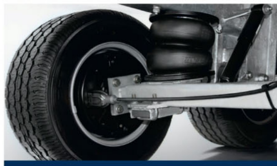
AIR SUSPENSION SYSTEM The trailer tilts automatically and the system is maintenance-free.
