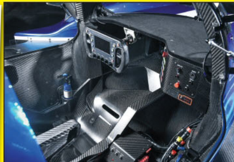
The carbon tub is a clever and lightweight design
