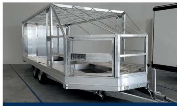
ALUMINIUM CONSTRUCTION Complete alloy chassis giving the system the lowest empty weight.
