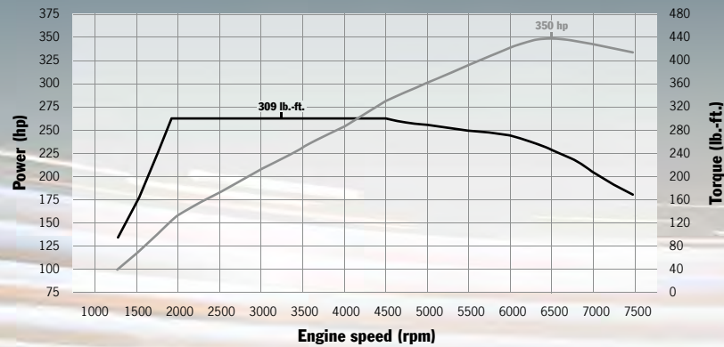
718 Boxster S and 718 Cayman S: 350 hp at 6500 rpm, 309 lb.-ft. between 1900 and 4500 rpm
