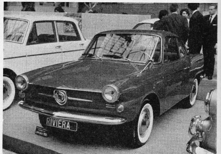
GERMANY is well represented at the Show, and this smart little machine is the Neckar. The car is, in effect, a German-built Fiat using the 767 c.c. rear-engined chassis with open and closed bodies.
