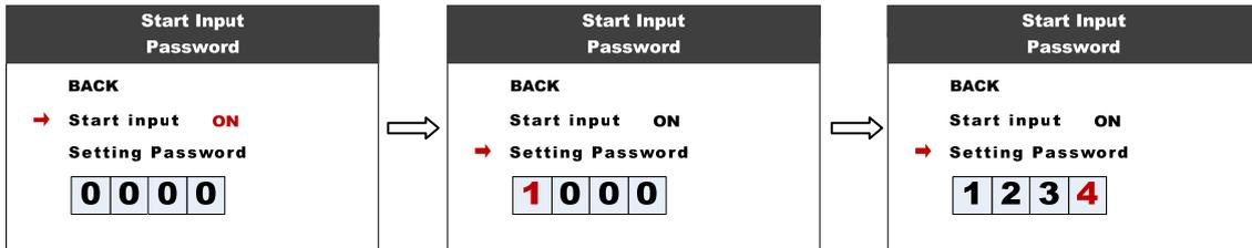
You need to input the right password before start with 30 seconds, display will power off automatically if the password was wrong three times.
