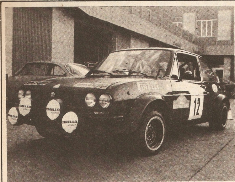
This is Autodelta's new Group 2 1500cc Alfasud that was launched on the recent Targa Florio Rally. The car, which although still on carburetors should change to fuel injection fairly soon, was driven by Federico Ormezzano and Bruno Scabini, who will be running the car in the Italian rally championship.
