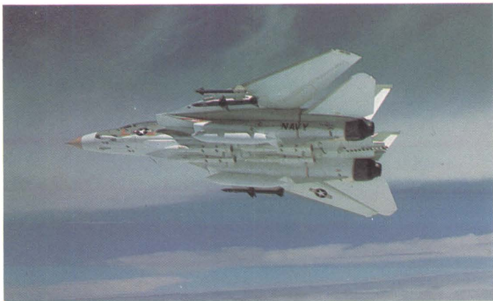
Above: Carrying tanks, this unusually painted F-14A is loaded with four Phoenix, two Sparrows and two Sidewinders.
