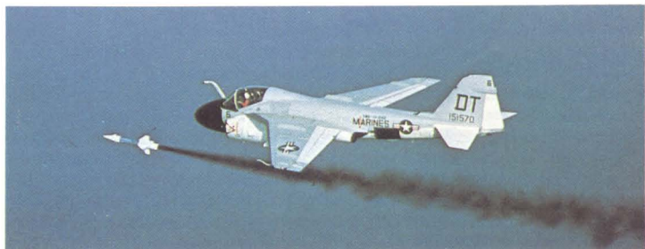
Above: Developed in 1950-56, the AGM-12 Bullpup was the first ASM (air-to-surface missile) to go into service after World War II.
