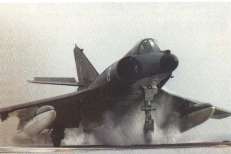
Above: Steam-catapult launch of the eighth Super Etendard, carrying the usual underwing tanks. Note the tailplane angle.
