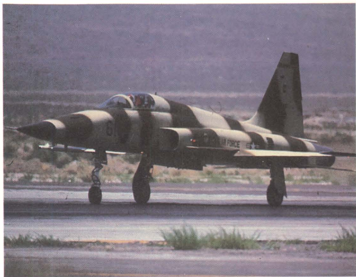
Above: Takeoff, probably from Nellis, of one of the Aggressor F-5Es used by the US Air Force. Together with similar aircraft of the Navy they have been used to evaluate at least 14 colour schemes to reduce air-combat visibility or to confuse the enemy as to attitude.
