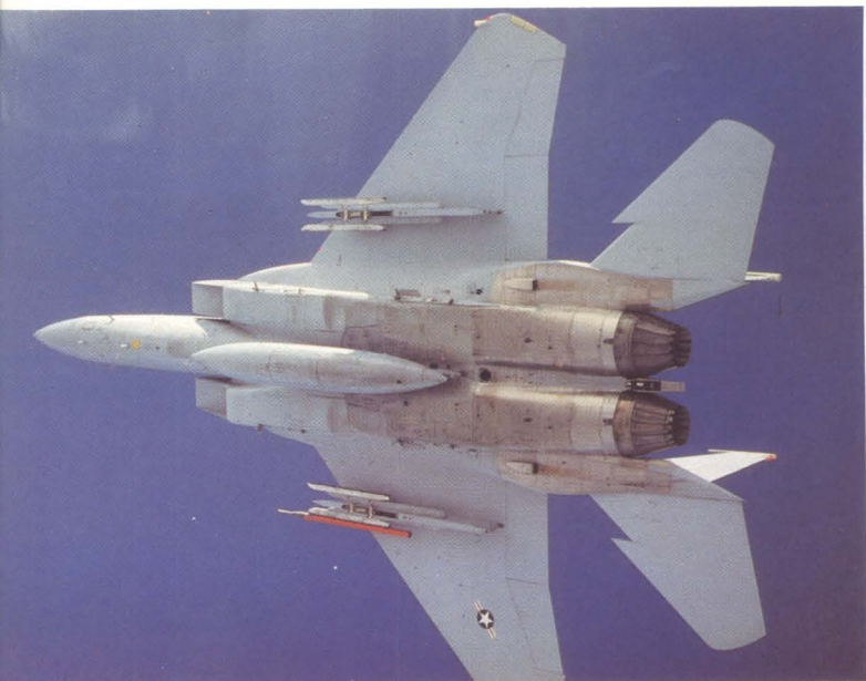
Above: An F-15C used for missile firing tests seen in clean condition apart from centreline tank and red instrumentation link.
