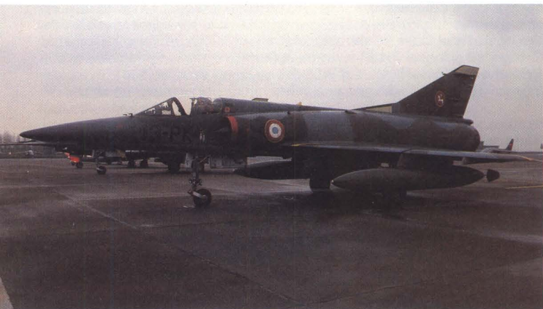
Above: One of the 20 Mirage 5F attack aircraft (originally built and paid for by Israel) which equip EC3/13 Auvergne at Colmar. This version has a longer and slimmer nose than the Mirage IIIs.
