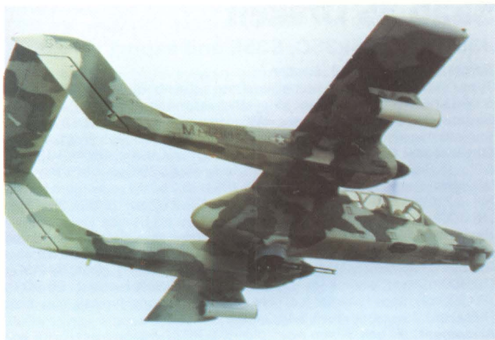
Above: This Marine Corps YOYV-10D prototype has now led to squadron deployment of 17 basically similar OV-10D Night Observation Surveillance aircraft with much new equipment.
