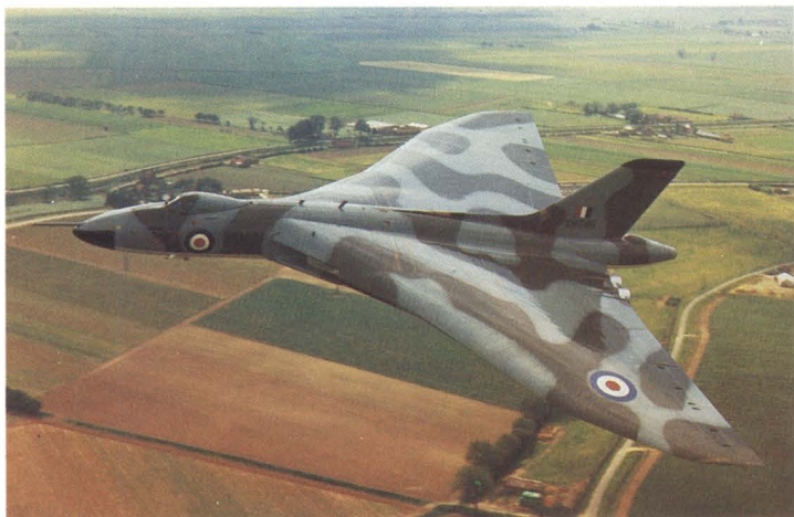
Above: A halcyon study of a B.2 taken in mid-1960s when low-level operations were new (passive warning and TFR are both absent).
