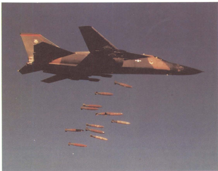
Above: Most 'Aardvarks' use only the four inboard pylons, and the basic design is such that the body cannot be used except for an ECM pod. Here 1,000lb bombs leave an F-111D.
