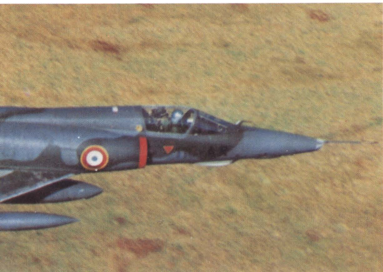
Above: One of the 20 Mirage 5F attack aircraft (originally built and paid for by Israel) which equip EC3/13 Auvergne at Colmar. This version has a longer and slimmer nose than the Mirage IIIs.
