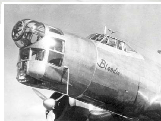
TOP & ABOVE The aircraft used for SIGINT/ELINT missions in 1946 was B 3A (Ju 86K-4) serial 150, named Blondie, powered by a pair of 820 h.p. Nohab My III (licence-built Bristol Pegasus III) radial engines. The cylindrical excrescence on the underside of the fuselage just aft of the mainwheels in the top image is the radome for its crucial AN/APS-15 navigation radar.
