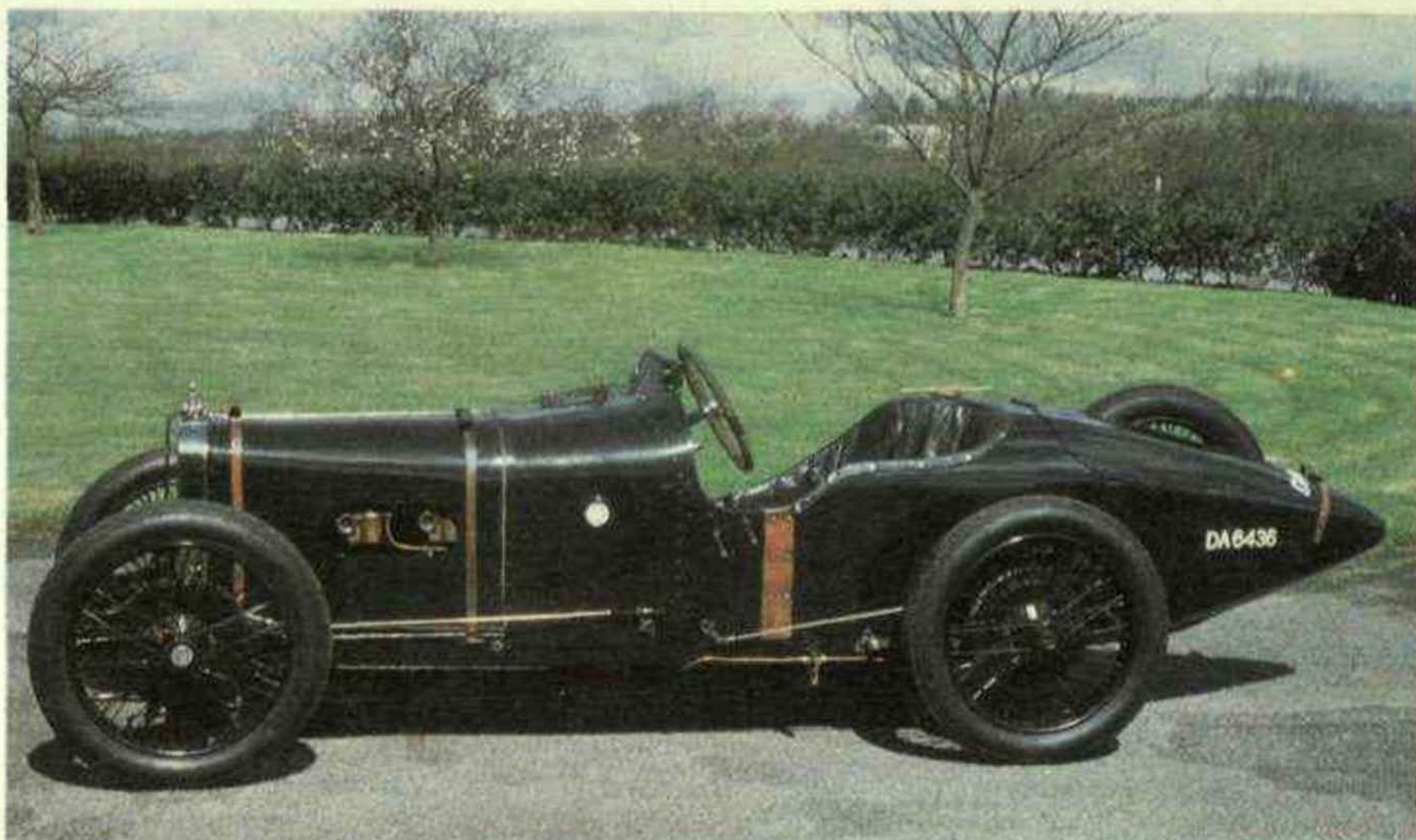
A n/s. view of the Sunbeam, showing the two carburetors, the staggered seating, and the joint in the two-section body. On the left, top to bottom, the engine, the 3-piece front axle, the stoneguard on the scuttle, a dashboard plate, and the partially-concealed spare wheel.
