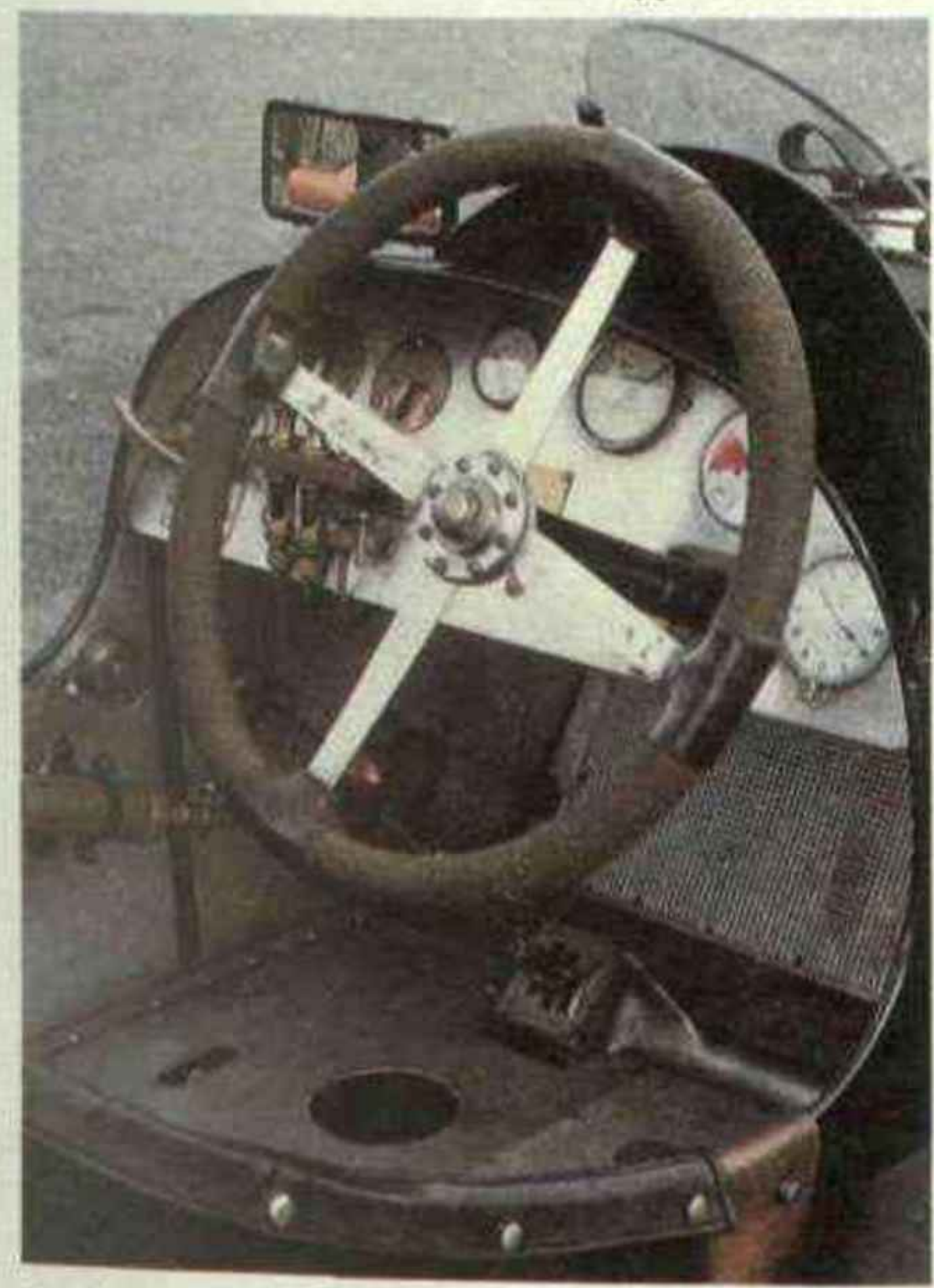
A cockpit view of the 1922 GP Sunbeam. The slot in the floor is for brake cross-shaft clearance, the hole for access to a tap to cut off oil seepage into the dry-sump.
