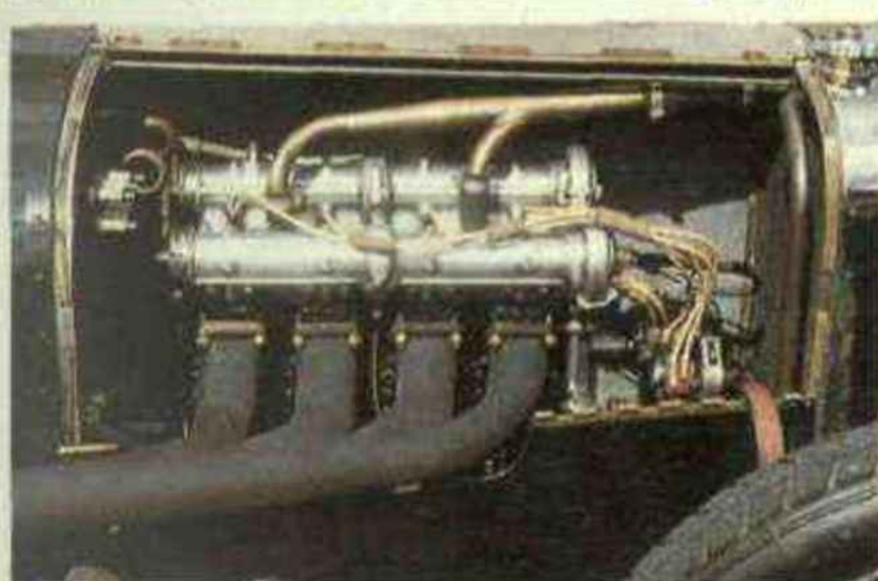
A n/s. view of the Sunbeam, showing the two carburetors, the staggered seating, and the joint in the two-section body. On the left, top to bottom, the engine, the 3-piece front axle, the stoneguard on the scuttle, a dashboard plate, and the partially-concealed spare wheel.
