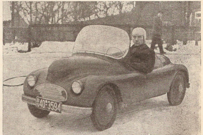
Yes, it is really meant to go on the road! Designer-constructor George Wolf in his "Little Wolf" (referred to on the opposite page). Weighing 418 lb., it is powered by a 200 c.c. air-cooled four-stroke motor and maximum speed is said to exceed 45 m.p.h. Fuel consumption is stated to be about 100 m.p.g.
