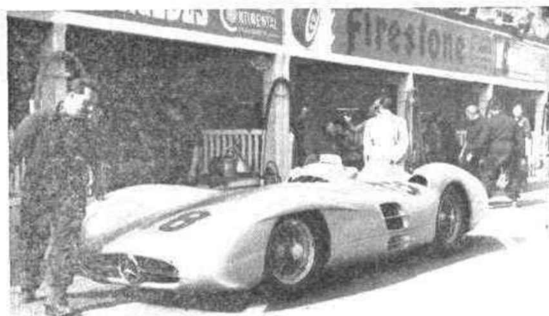
WINNER FIRST TIME.—Fangio's Mercedes-Benz seen during practice at Reims. The mechanic illustrates the low build of the car, in spite of its large plan-area. In front of the rear wheel is seen one of the scoops for cooling the tyres, while for race-day the chromium star and cross-brace were removed from the nose of this car.
