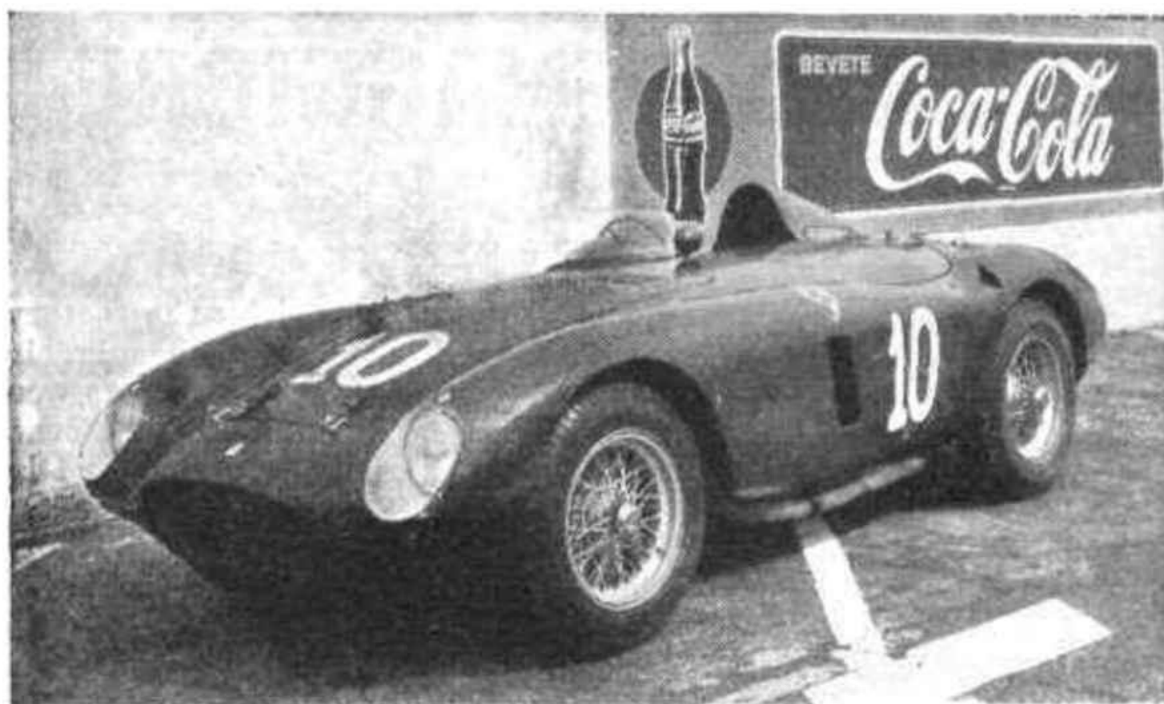
THE NEW 750S FERRARI sports model, a 3-litre four-cylinder with the same design of engine as the 1954 Formula 1 car. This one finished second in the G.P. Supercortemaggiore, driven by Gonzalez and Trintignant, but a week later it failed to last the 12-hour race at Reims due to trouble in the transmission.
