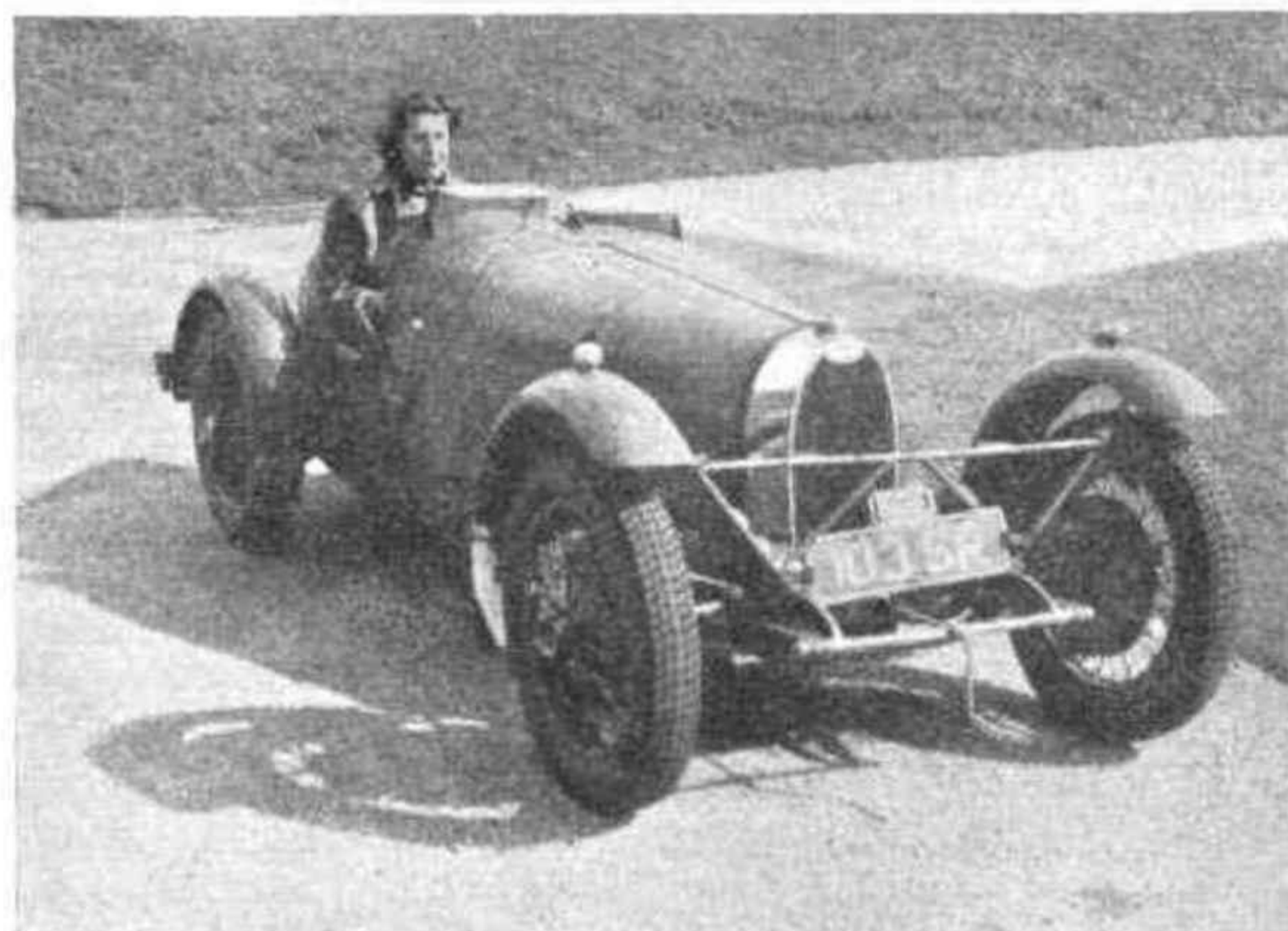
TYRO.—Averil Scott-Moncrieff in her first Bugatti, a Type 37A supercharged, single-cam, four-cylinder G.P. car.
