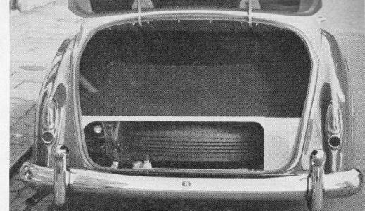
AMPLE luggage space as well as an accessible spare wheel and cleverly placed tool compartments (to the left of the spare wheel with lined box above) are among the things automatically provided on a car of the quality of the Bentley.
