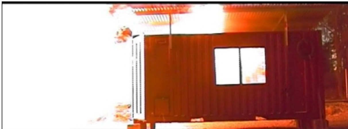
Figure 7. The unburnt gases are combusted in a dramatic fireball outside the container.
