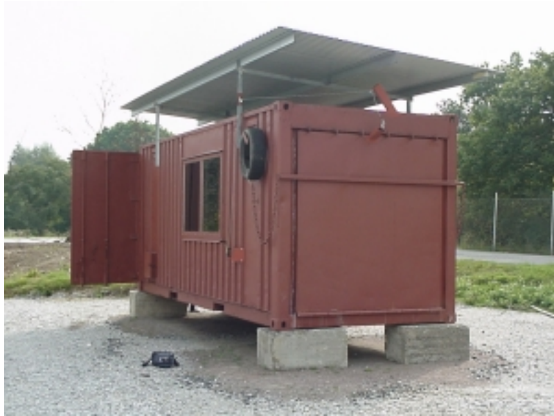
Figure 1. The pressure relief panel in closed position at the container's short side.
