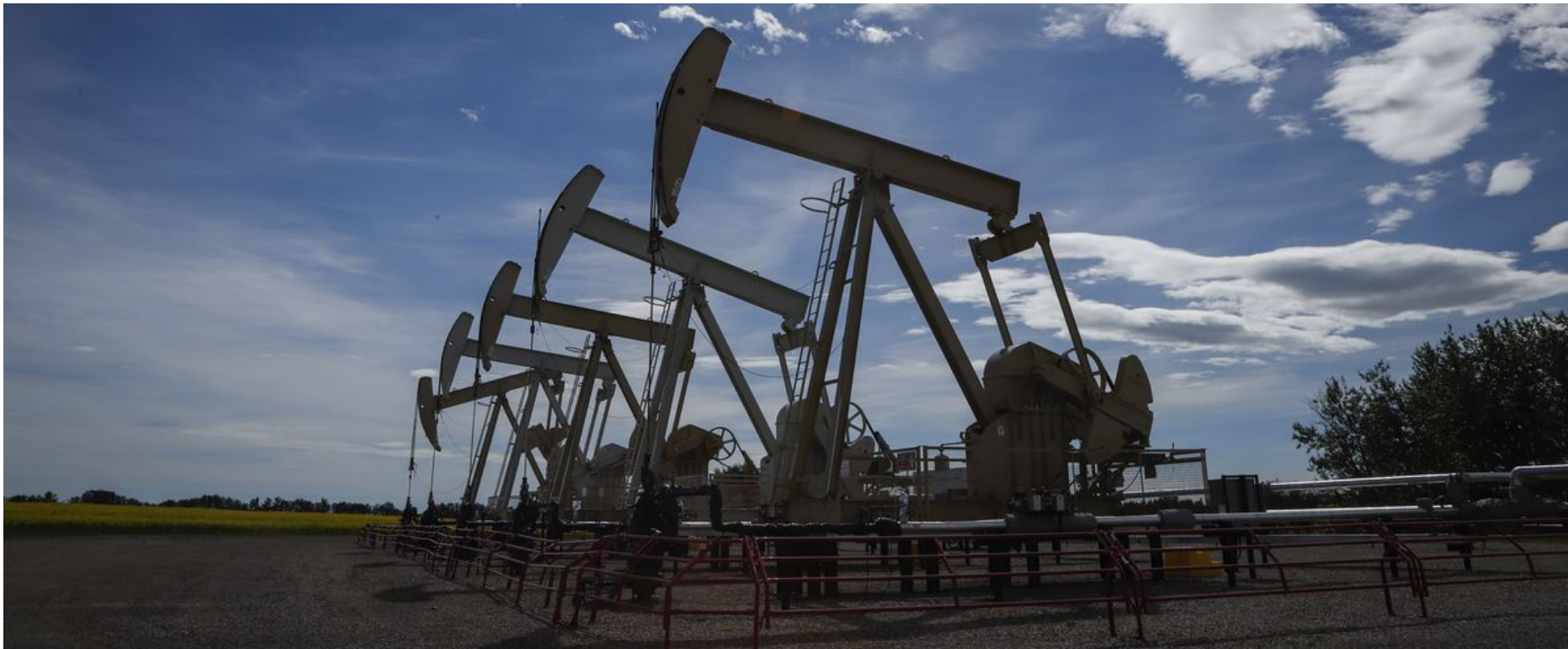
Pumpjacks draw oil out of the ground near Olds, Alta., on July 16, 2020.
