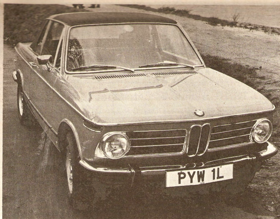
BMW 2002 Cabriolet's detachable roof with rollover bar does not affect rigidity.
