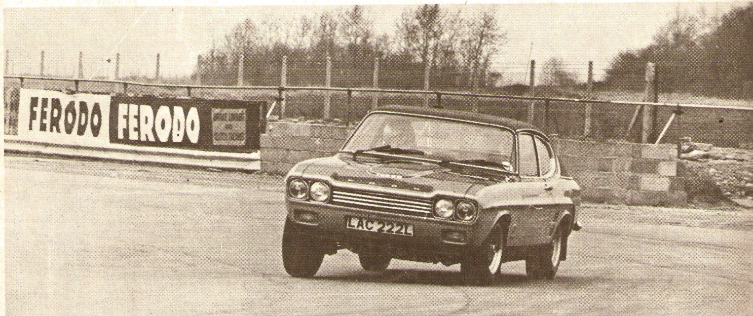
Open the throttle in a corner in the Broadspeed Bullit, and the handling characteristic changes progressively from understeer to oversteer as the turbocharger comes on strong.
