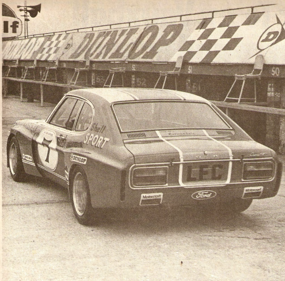
Main visual change on the 1973 Group 2 Capri is the neater, more aerodynamic wheel arches.
