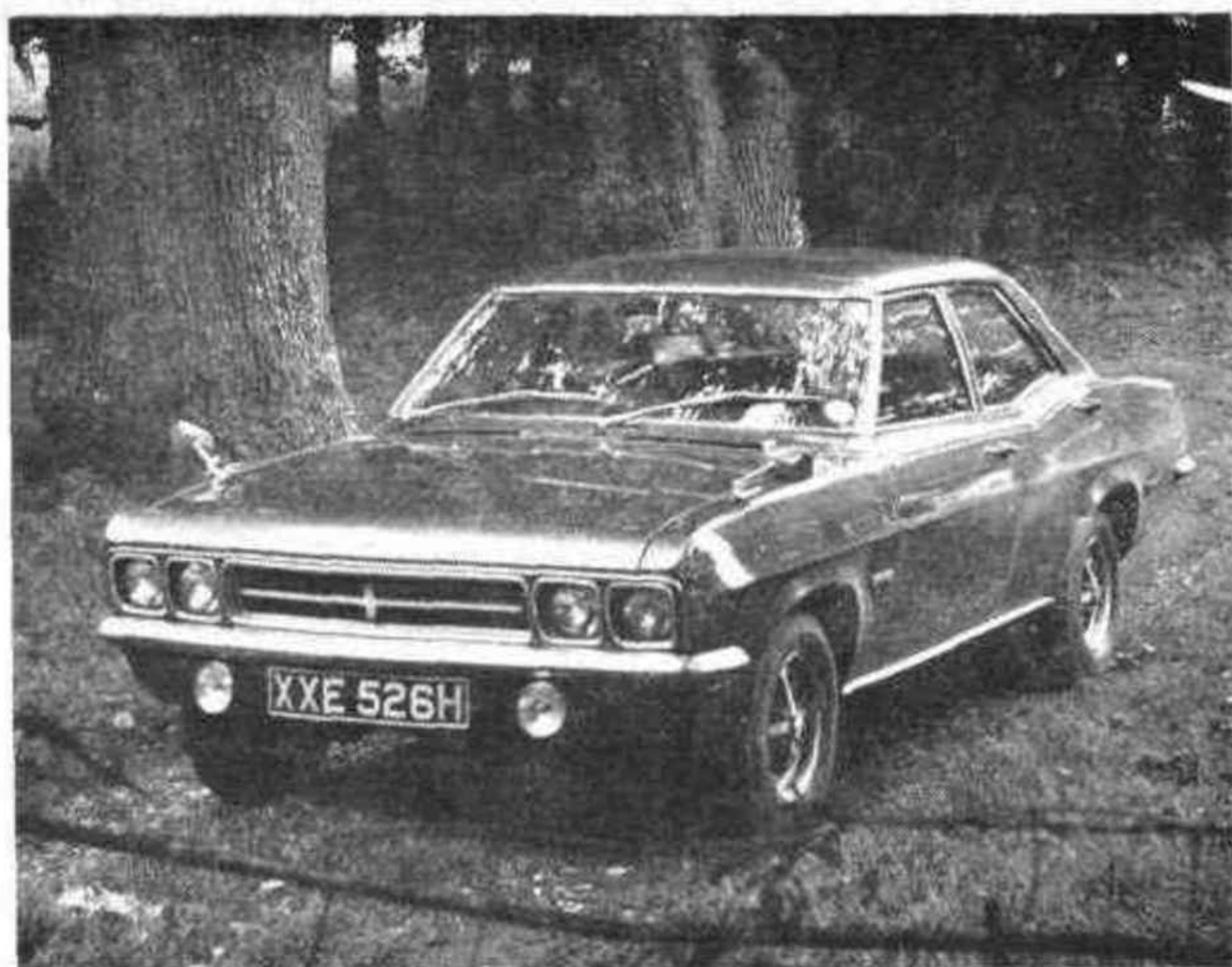
The Vauxhall VX 4/90 makes good use of a 2-litre o.h.c. engine in a Viva body shell but its handling is in the family-saloon category.
