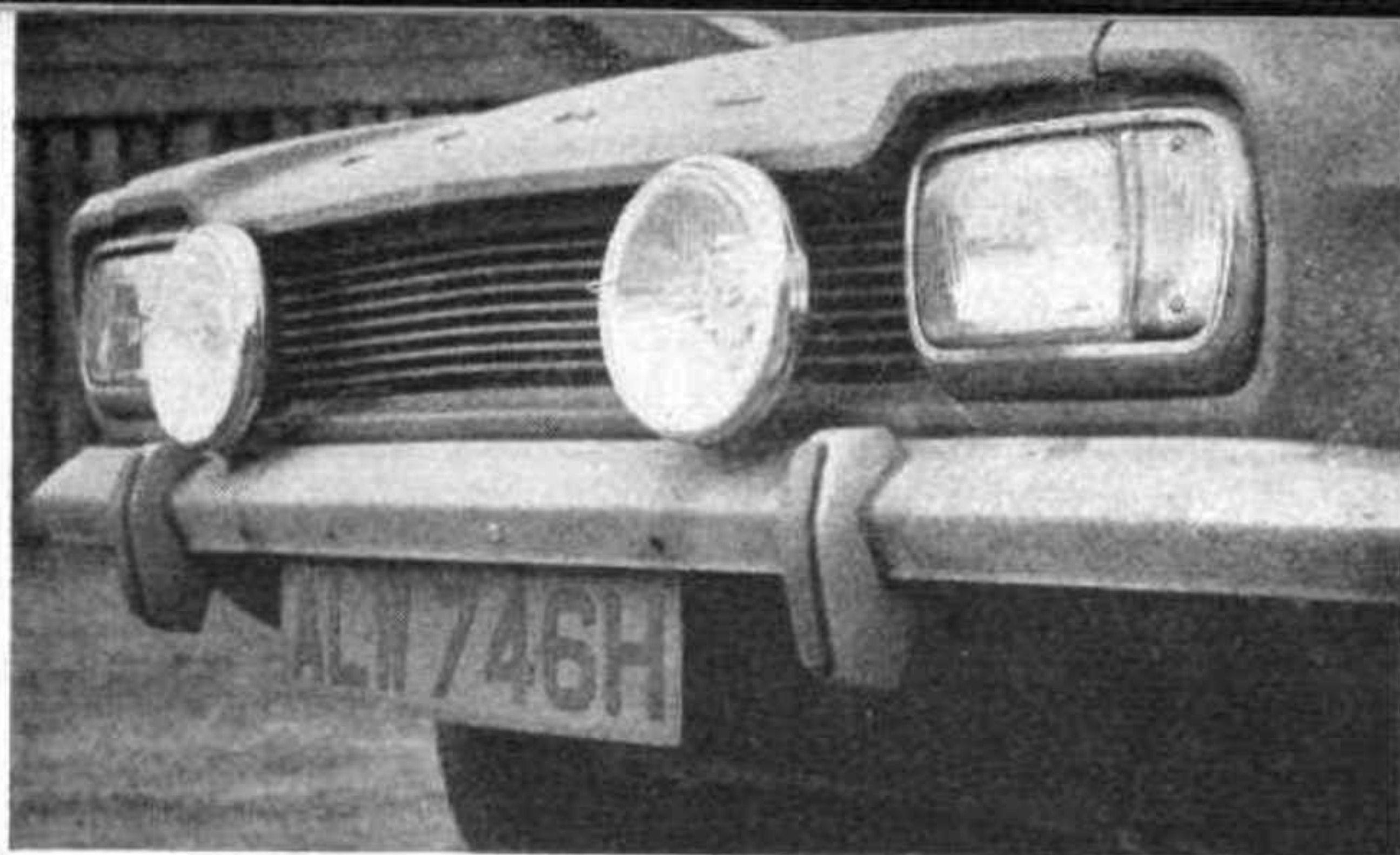
CONVERSION —these Starlux Marchal lamps were not intended to fit the Capri, so some brackets were fabricated to keep the owner a lot happier about seeing the way ahead.
