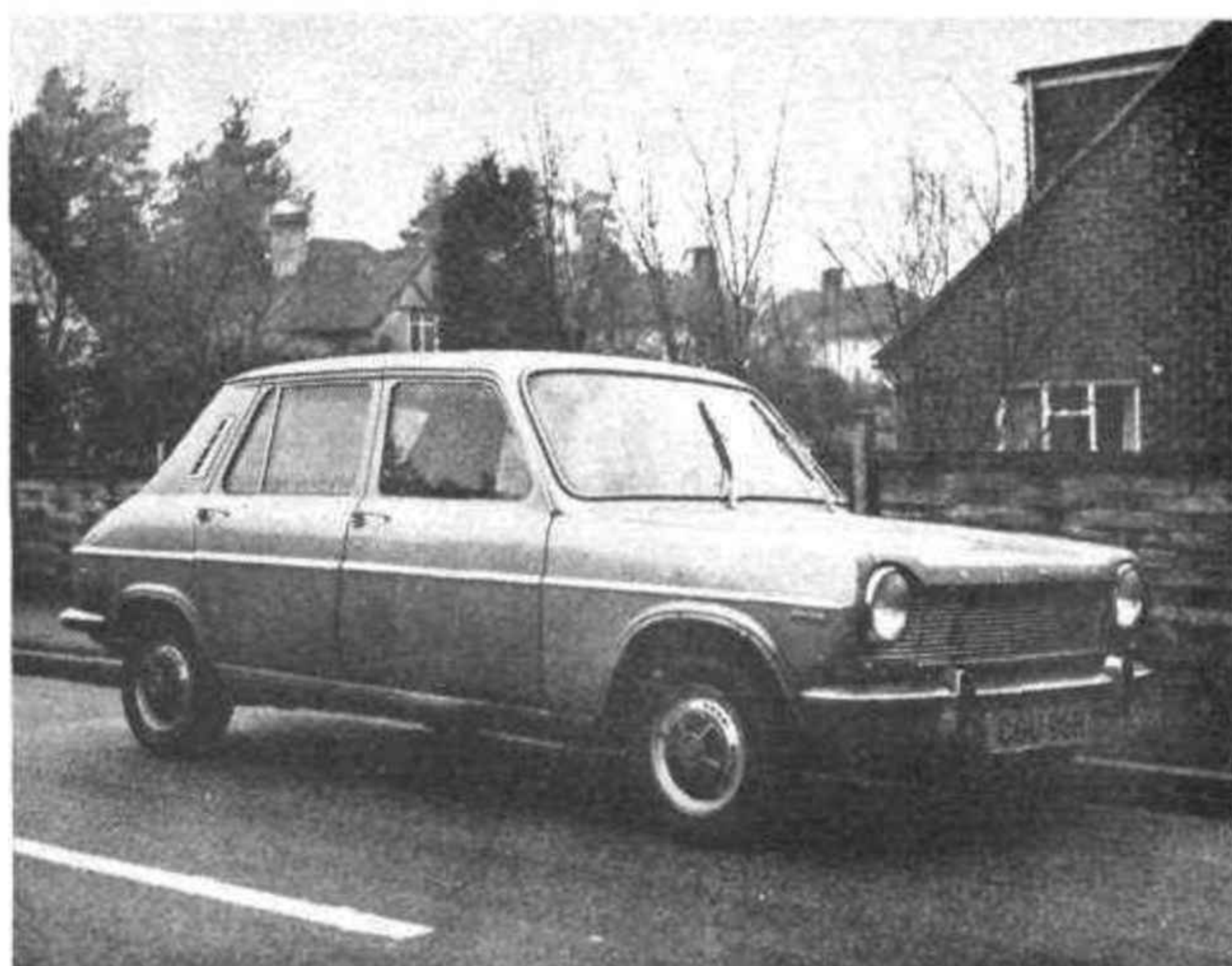
The Simca 1000 GLS is an exactingly nice small car, with sensible five-door bodywork and front-drive from a transverse engine, but the noise level is high.
