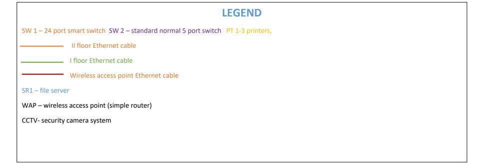
Every PC on the II floor is connected to the SW 1 (24 port smartswitch), every printer is connected to PC next to them (they don't have Ethernet ability, older printers). Every PC has its own static IP address. All PCs on first floor are connected to switch 2 (5 port) which is connected to switch 1 (24 port) by Ethernet cable trough wall socket. CCTV security camera system needs just internet connection and it can have dynamic ip address.
