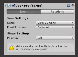
The door script has 2 tabs, the *Door Tab* and the *Rotations Tab*. In the door tab, you need to select what type your door is. Select whether or not the scale correctly matches with Unity3D units, and also select if the pivot position is centered or correctly positioned. To see whether the pivot position is centered or not, make sure the tool handle is places at the active object's pivot point. You can do this by toggling this:
