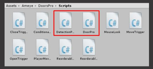
The door tool itself comes with 2 main scripts, 'DoorPro' and 'DetectionPro'. You can find them under Assets>Ameye>DoorsPro>Scripts. Drag the detection script onto the player you just created and then drag the door script onto every single door in your scene. When you drag the door script onto your door, it will automatically create a hierarchy around the door model. There will be a parent object added to your door model and later on also some children.
