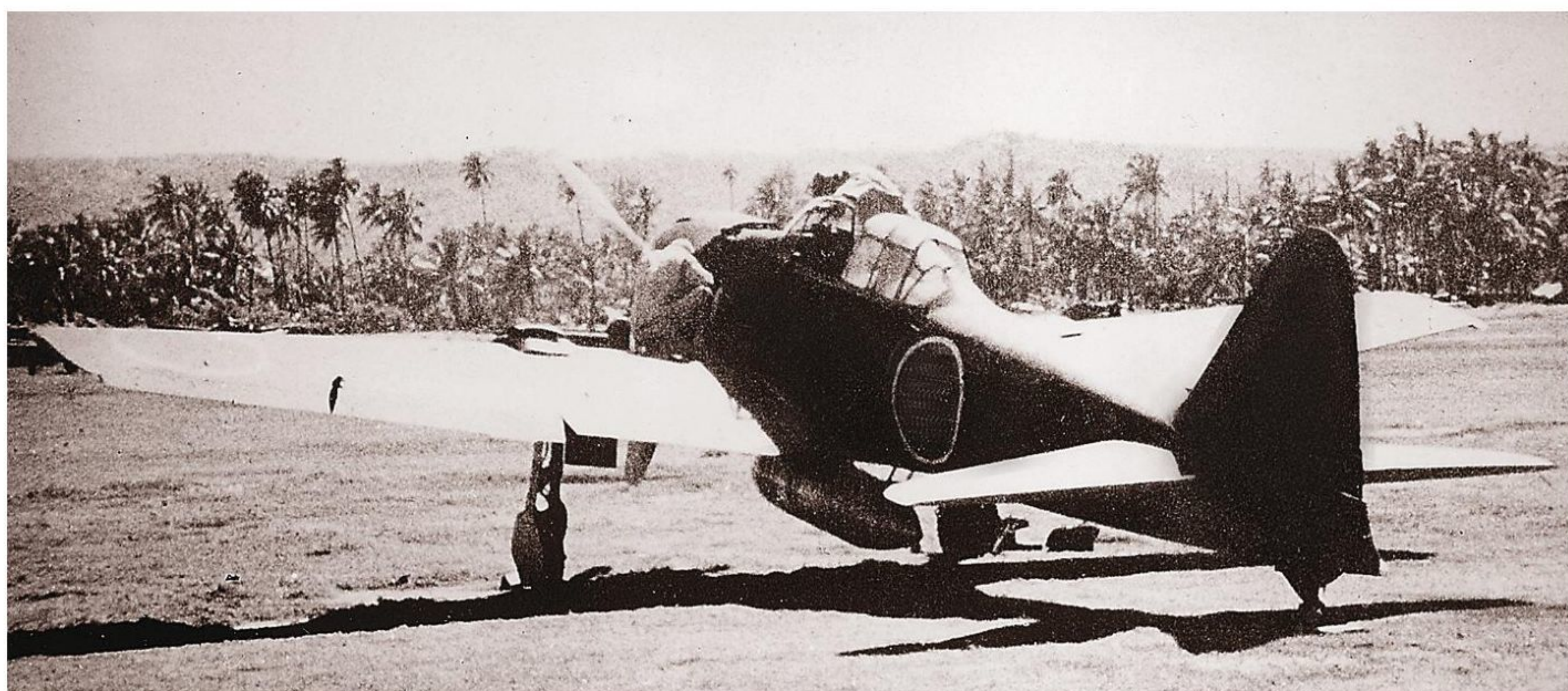
A clipped wing version of an A6M Zeke 32. (Photo courtesy of Peter M. Bowers collection.)
