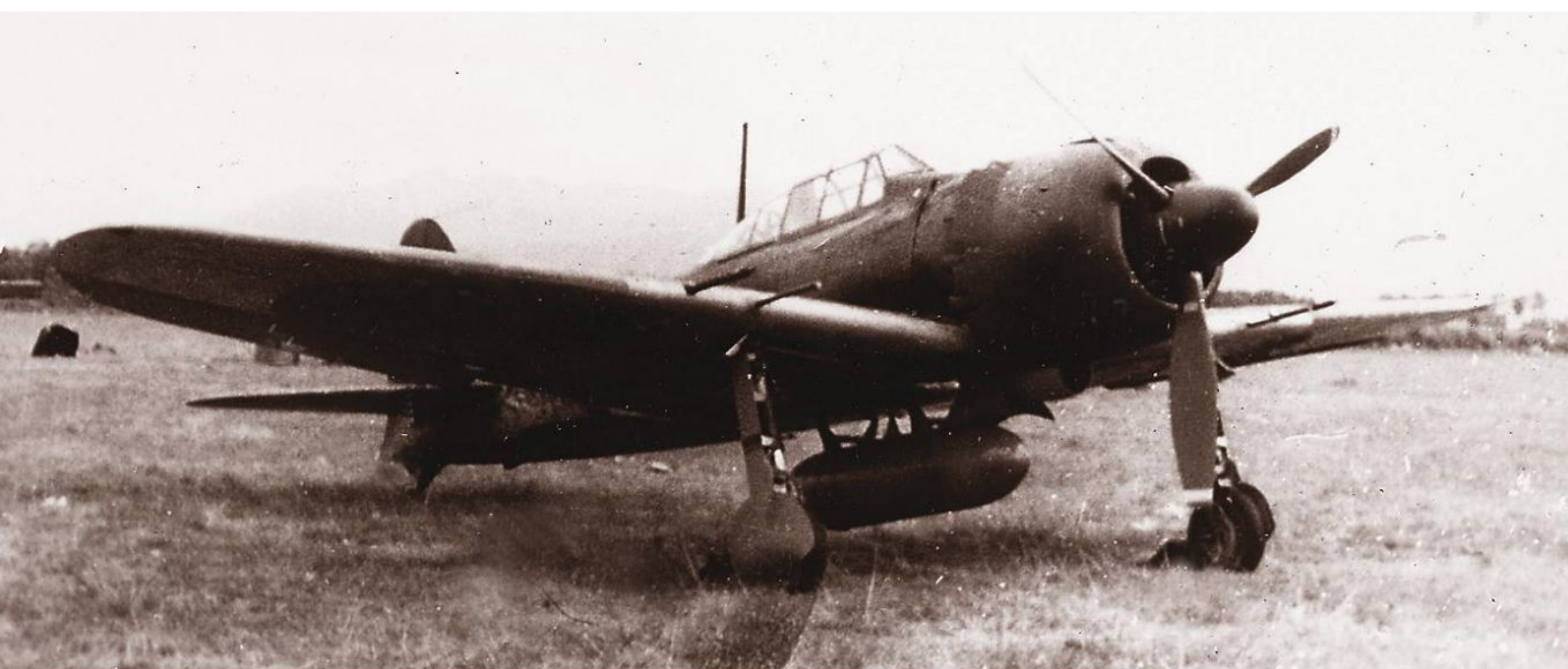
An A6M5 with cannon and auxilliary fuel tank. (Photo courtesy of Peter M. Bowers collection)
