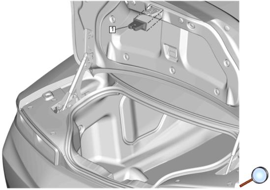
1. Use a small flat-bladed tool to pull and release the rear compartment latch cover (1).
