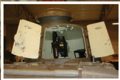
Left: The rotating turret did not accommodate a hatch; therefore, the commander's field of vision was limited to that afforded from a small cupola
