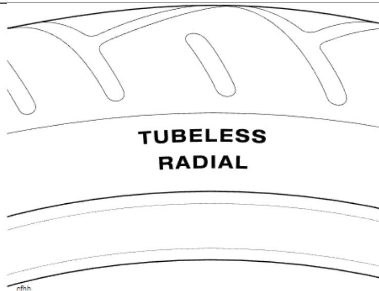
Typical Tyre Marking -Tubeless Tyre
