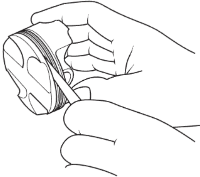
Piston Ring-to-Groove Clearance Check
