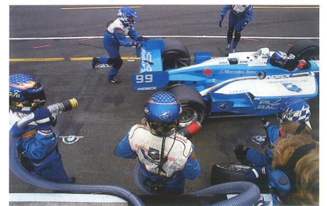
12-14 Seconds: When the vent man sees fuel in his window he pulls off and this signals the fueller to pull out. This is the most dangerous part of the stop, as it is important to get clear of the car. Rear wheel changers may push the car away and a jet of water is shot at the fuel filler on the car to clean away any residue."
