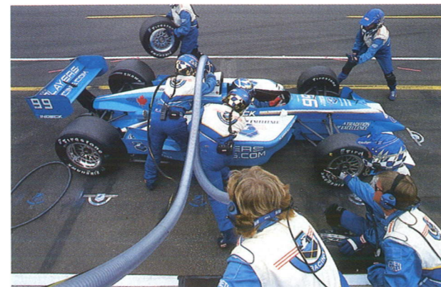
8-10 seconds: The car should be on the ground now and in gear. This is most nerve-racking time as we now only wait for the fueller and the vent man . If the front wing needs adjusting, this is by the front wheel men. Fuelling continues. Farside front wheel man takes job of holding the car until stop completed."
