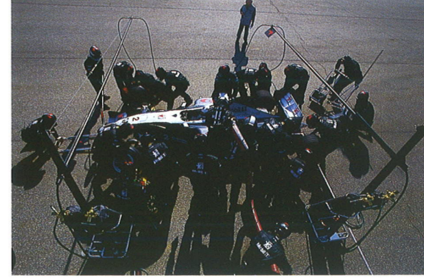
2 - 3 Seconds: The wheels are taken off the car. The mechanics with the air hammers have a spare wheel nut in case there are problems with the original one. A second mechanic removes the wheel from the hub. Refuelling continues."
