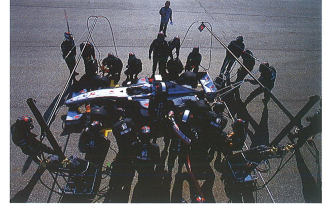
6-7 Seconds: Fuelling about to finish. The driver is shown the 1st. Gear board, and as soon as the required amount of fuel has gone into the car, the hose is off. The driver gets the signal to exit."
