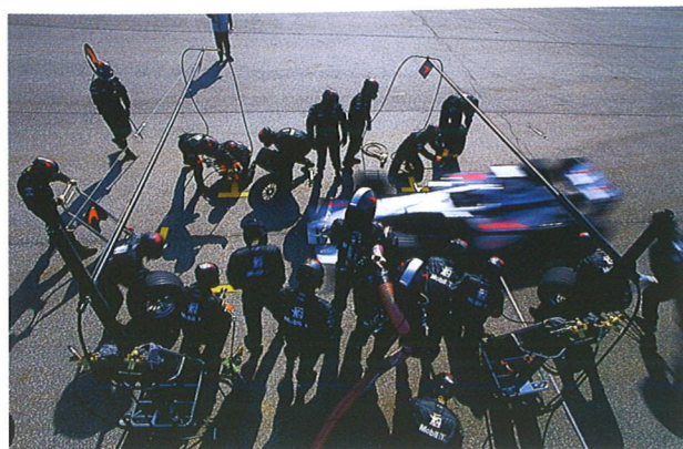
Minus 30 seconds Tyres taken out of tyre warmers. Pit crew assembles in pit lane. The car arrives having slowed from the 50mph pit lane speed limit. The lollipop is placed in front of driver to show him where to stop."
