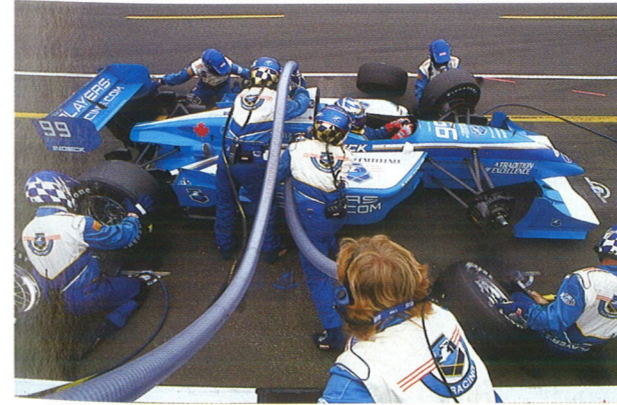
2 - 4 Seconds: The old tyres are taken off - actually, the wheel nuts should be off within two seconds, and then the wheels are removed. The new tyres are put on and the fuelling continues. The fuel hose holds five to six gallons and is therefore quite heavy - I guess the total weight is about 45 pounds."
