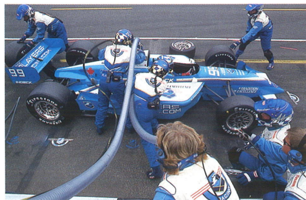
6-8 Seconds: By now all wheels should be OK. It should take about 6.5 seconds to change the outside rear wheel as the guy had to run around the back. Farside front wheel man throws wheel gun and air line to colleague over the wall to clear the way for the car's exit. Refuelling continues."
