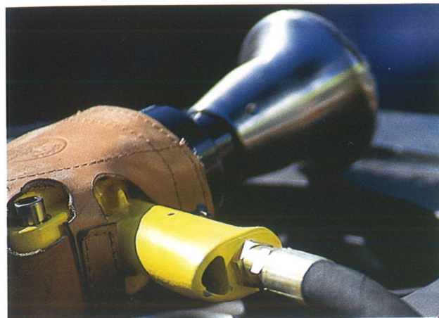
Above left: The McLaren wheel man carries a spare nut just in case of problems. Above right: The hammers are operated by compressed air
