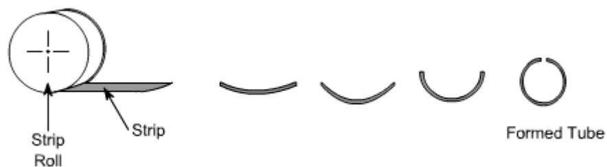
Fig 11.10: Forming of Tube from Strip
