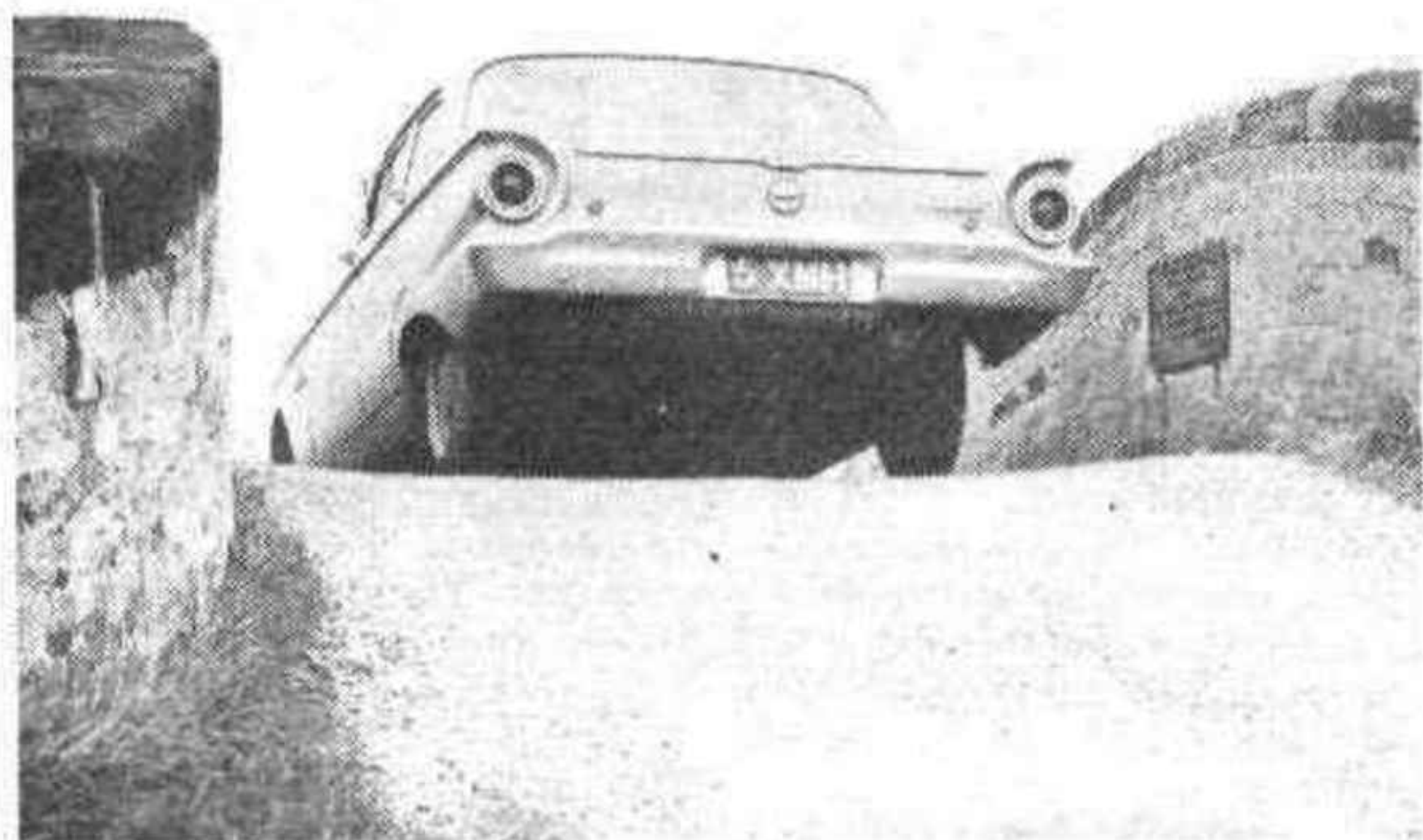
TIGHT SPOT, even for a "compact." This unusual view of the Ford Falcon well illustrates the treatment of the rear-end, with large rear window, recessed lamps and absence of tail-fins.
