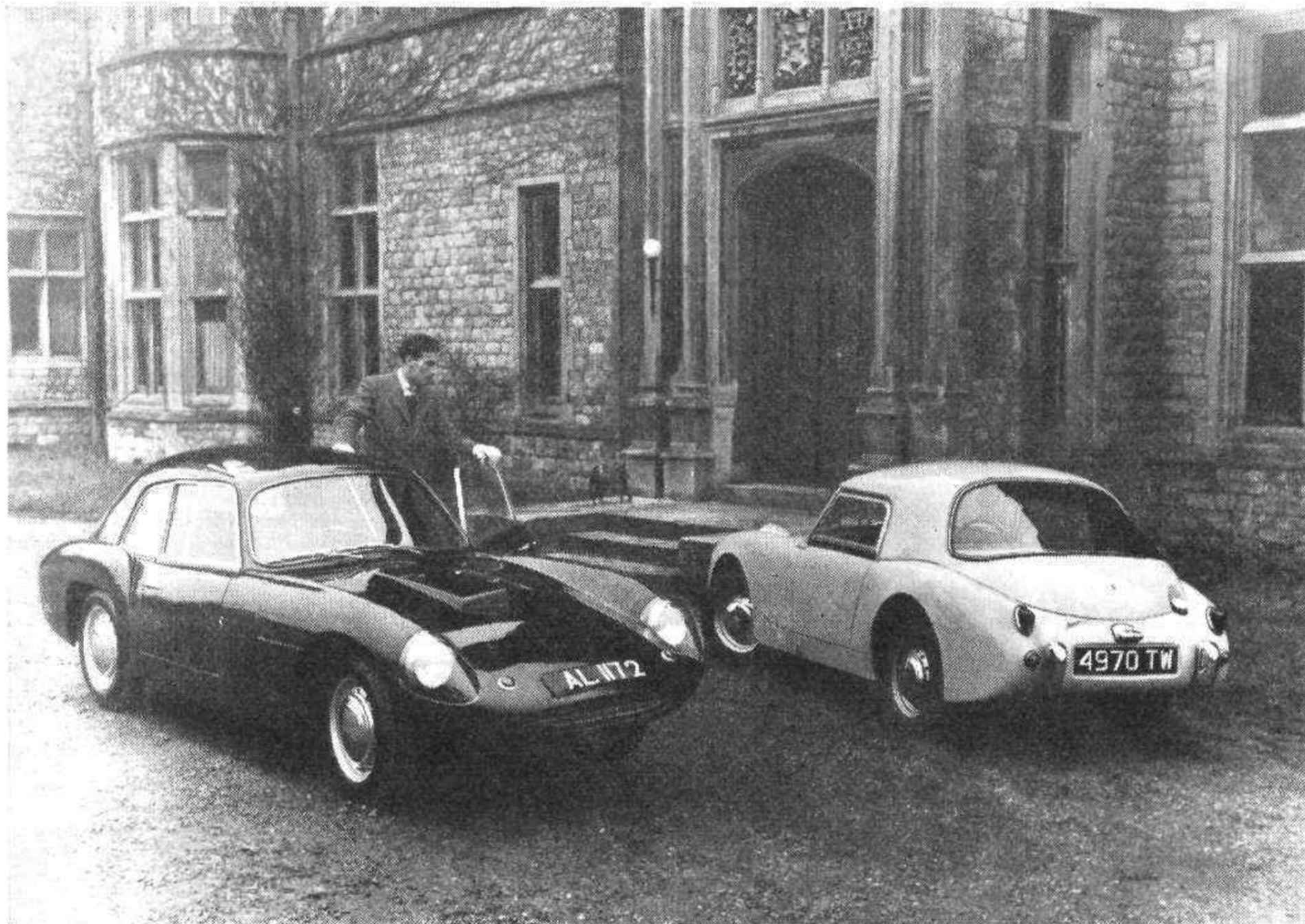
The 1172 fixed-head coupé mounted on a Ford chassis and a Sprite fitted with G.T. Hard-top.
