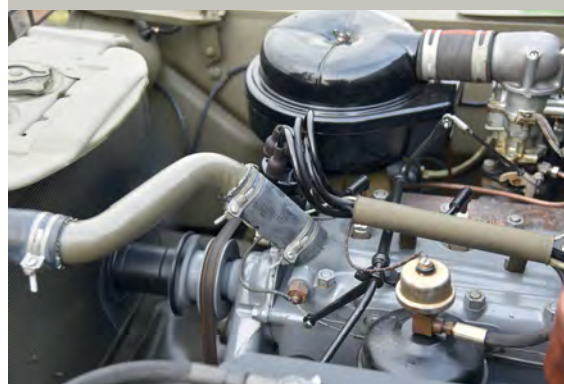
The GP's four-cylinder, sidevalve engine is derived from the Fordson Model N tractor unit
