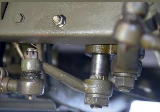
The second steering box is mounted to the chassis in front of the rear axle
