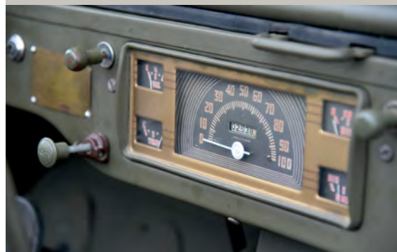
The Ford GP used the instrument panel from the 1941 civilian Ford pick-up
