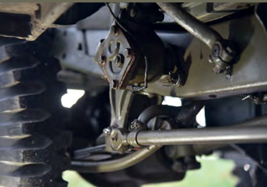
The front steering box has an extra linkage to connect to the secondary one
