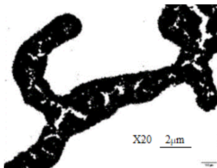
Figure 4. Floc image after IPP treatment.
