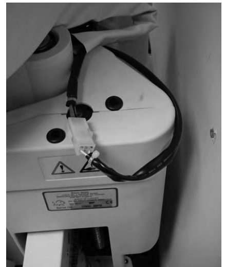
EXCESS WIRING IN TOP OF MAINFRAME
