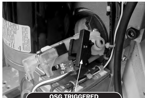
OSG TRIGGERED OSG Regulator weight in upright position
