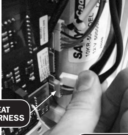
REMOVE TIE-WRAPs SECURING THE INTERLOCK HARNESS IN POSITION
