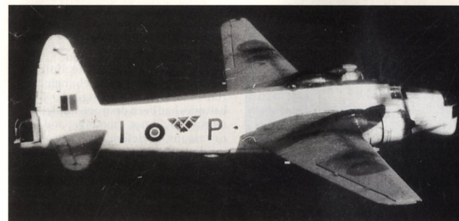
ABOVE A Wellington XII of 172 Sqn off the Taw Estuary in August 1943. This type had the retractable Leigh Light as well as ASV radar in a chin radome instead of the aerial array above the fuselage.
