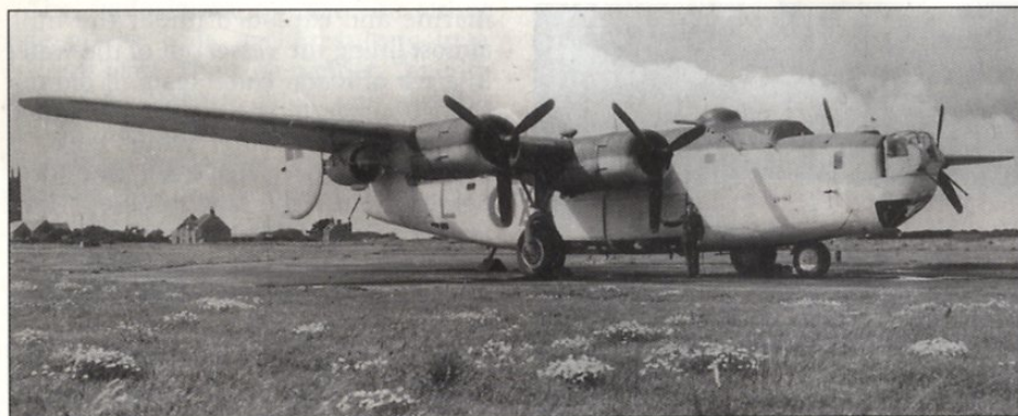
LEFT A Consolidated Liberator VI at St Eval, Cornwall, with a nacelle-type Leigh Light under its starboard wing.
