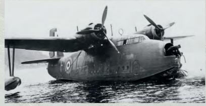
"Lerwicks could not maintain height on a single engine... Hydraulic failures caused the bomb doors to droop open... Excessive corrosion was found around the rear turret, due to ingestion of spray"
