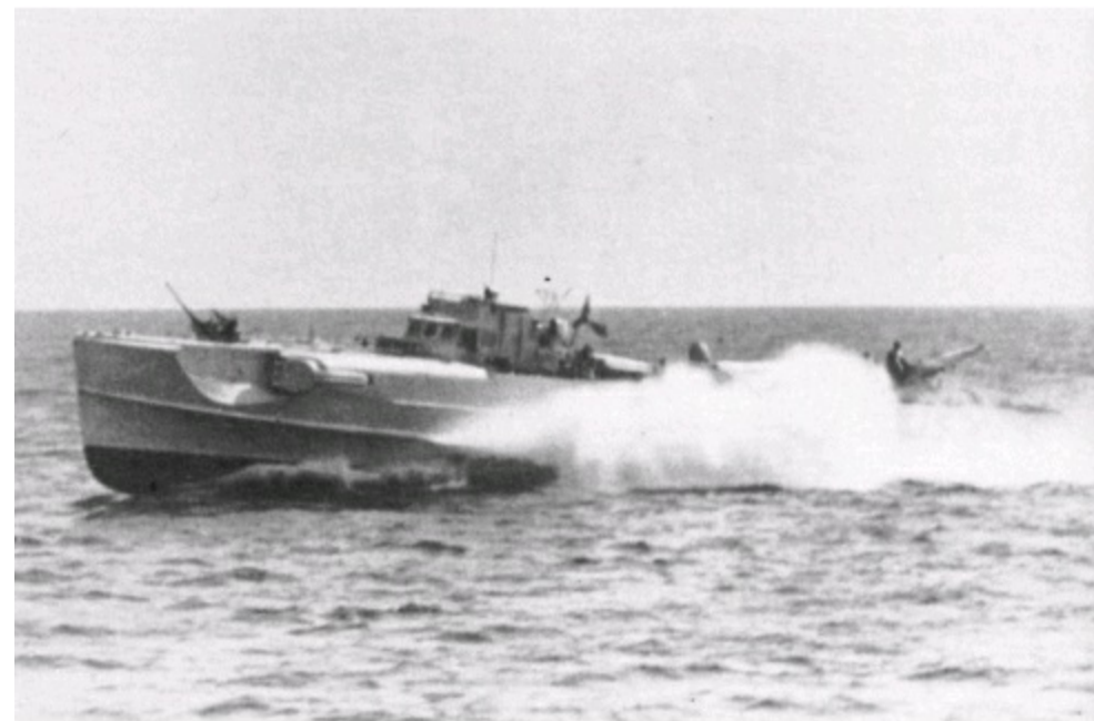
One of the smaller 82-ton E-boats, S.81, built by Lürssen in 1942 and showing the familiar built-in torpedo tubes with the armoured 'cupola' shaped bridge and 20mm AA guns forward and aft. The forward gun could be raised or lowered through a manhole. Although able to achieve a maximum 36 knots, the E-boats remained nearly horizontal in the water and did not lift their bows in the same manner as the planing craft of the British and American forces
