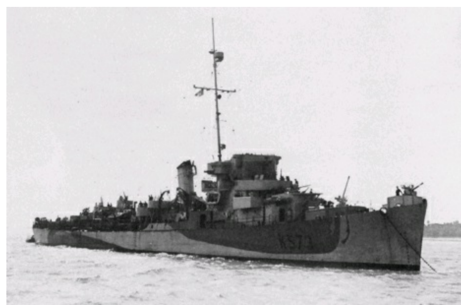
HMS Stayner, one of the US destroyer escorts built in 1943 for the Royal Navy which was specially equipped for anti-E-boat work, including surface radar and a 2-pounder bowchaser
