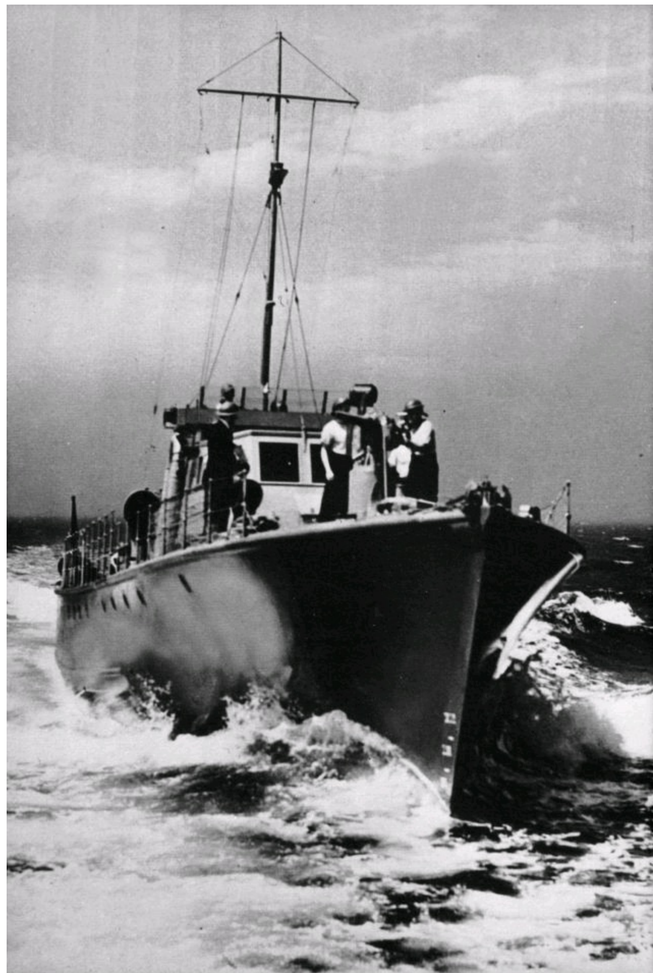
A Fairmile 'B' motor launch, built in Canada for the Royal Canadian Navy and used for anti-submarine patrols in the St
