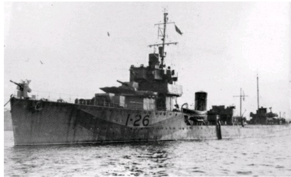
HMS Watchman. one of the First World War destroyers modified for escort duties. Armament included two 4inch guns, three 2-pounders, and two 20mm AA guns. To the left of the mast can be seen the special 'Headache' equipment for monitoring radio transmissions between E-boats. The 'bowchaser' 2-pounder gun provided close-range defence against E-boats.
