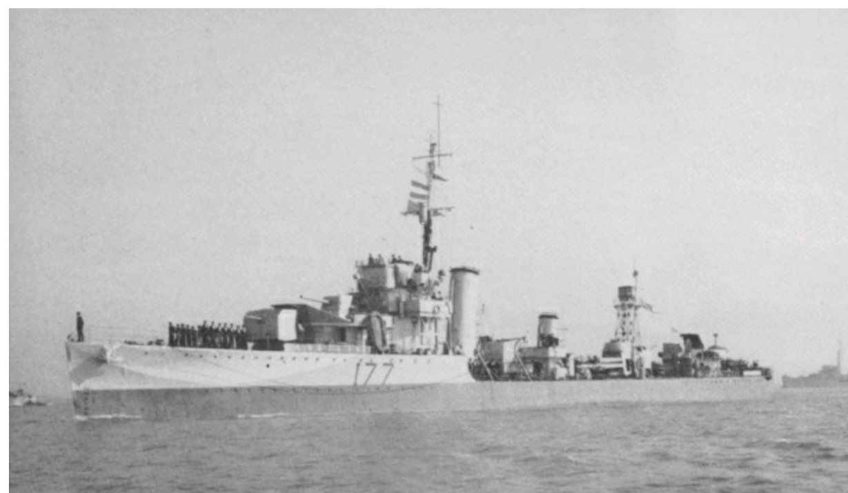
Another of the old RN destroyers modified for coastal escort duties, HMS Whitshed was further adapted in 1944 for anti-E-boat work when a twin 6-pounder replaced one of three 4.7inch guns and radar was installed so that MGBs could be vectored on to E-boats
