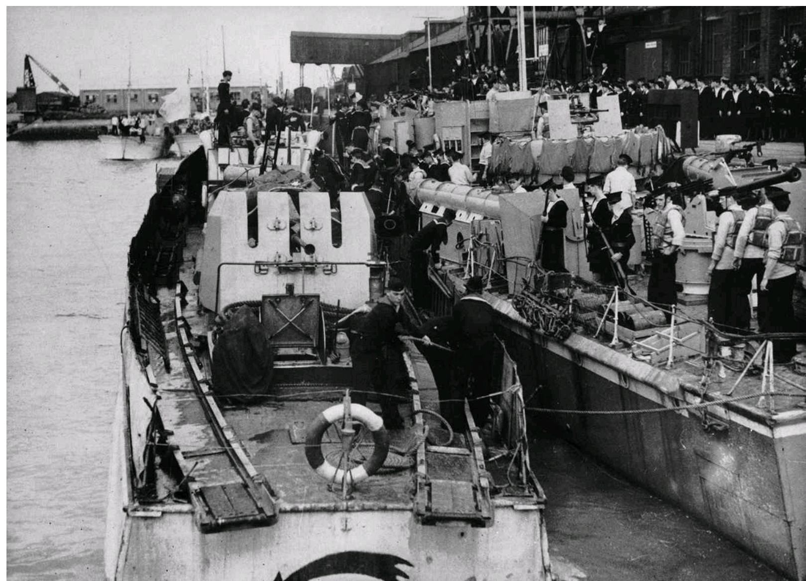
A surrendered German E-boat ties up alongside a Fairmile 'D' in Felixstowe harbour at the end of the war. The 37mm AA gun on the after deck was added to the larger types from 1944 onwards, and the rails on either side carried spare torpedoes or mines which were released from the stern
