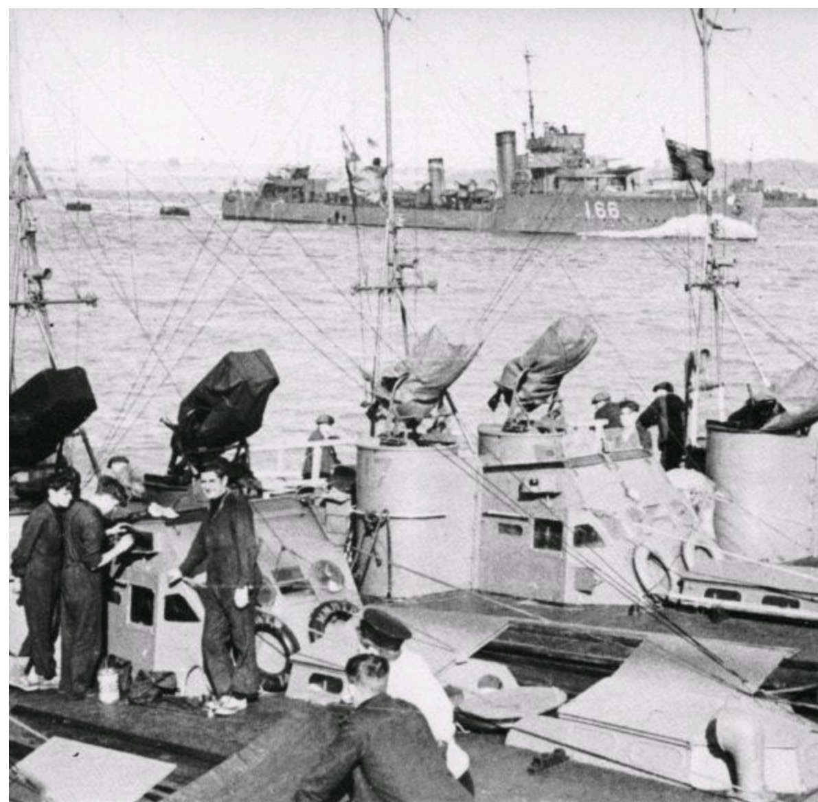
The original British Power Boat Co 60 ft 3 ins MTBs, built between 1936 and 1939 and formed into the 1st MTB Flotilla, first stationed at Malta but brought back to England in early 1940 as the nucleus of Coastal Forces, The quadruple .303inch machine-guns were originally in cockpits forward and aft, but were soon moved to wing positions on either side of the bridge, as can be seen here at Harwich in 1940. In the background is HMS Wivern, one of the Royal Navy's old destroyers which were modified for short-range escort duties until new ships were available
