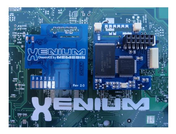
The Xenium has been designed to cater for a variety of installation options including Pin Header, Quick Solder, Hard Wired and Solderless methods.
