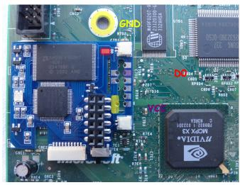
Again the process is exactly the same for console versions 1.4 and 1.5, the DO location is the same as versions 1.2 and 1.3. But for this installation I have shown the extra points required for a version 1.5 console, continue to use Kynar Wire with the aid of flux.
