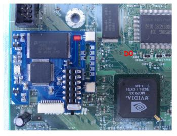
The process is exactly the same for console versions 1.2 and 1.3, the only difference is the top side DO location. However I would highly recommend the "Pin Header" installation method for motherboards that don't have the LPC filled with solder like the version 1.0!
