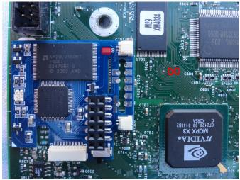
Place the Xenium mod-chip in place as shown above making sure it sits nicely in between all the components that surround it. While using flux, solder the pads on the Xenium to the LPC creating a nice little bead. Depending on your board you may need to scratch the solder mask of the top of the DO point shown above or use the alternate DO underneath the motherboard and connect it to the Xenium with Kynar Wire.
