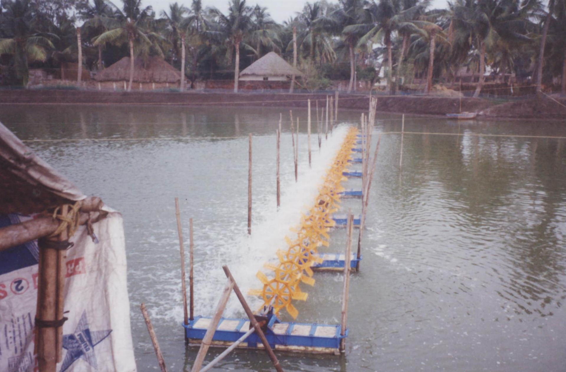
Commercial pond culturing Tiger Prawn in freshwater using long arm paddle wheel aerator (Farmer : N. Tejopati Rao)
