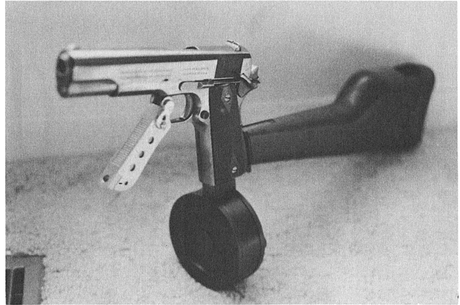
Same gun as viewed to the left, but this one has the Browning Hi-Power stock substituted. During testing, it was found the Hi-Power stock is far superior in design and function than the Lebanese type. The Lebanese stock latch that locks the stock to the main-spring housing of the gun tends to disengage easily during firing.
