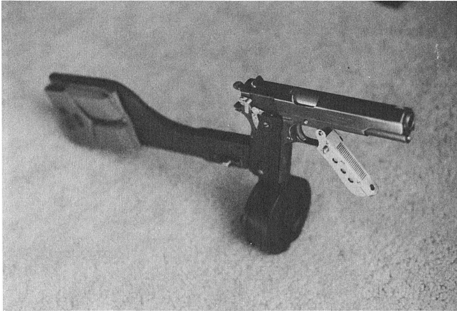
Perspective frontal view of the new Colt .45 machine pistol. This one has the Lebanese-issue, detachable shoulder stock and the 30-round Bingham snail drum magazine for ultimate firepower. Note the two pocket magazine pouches riveted to the shoulder stock.
