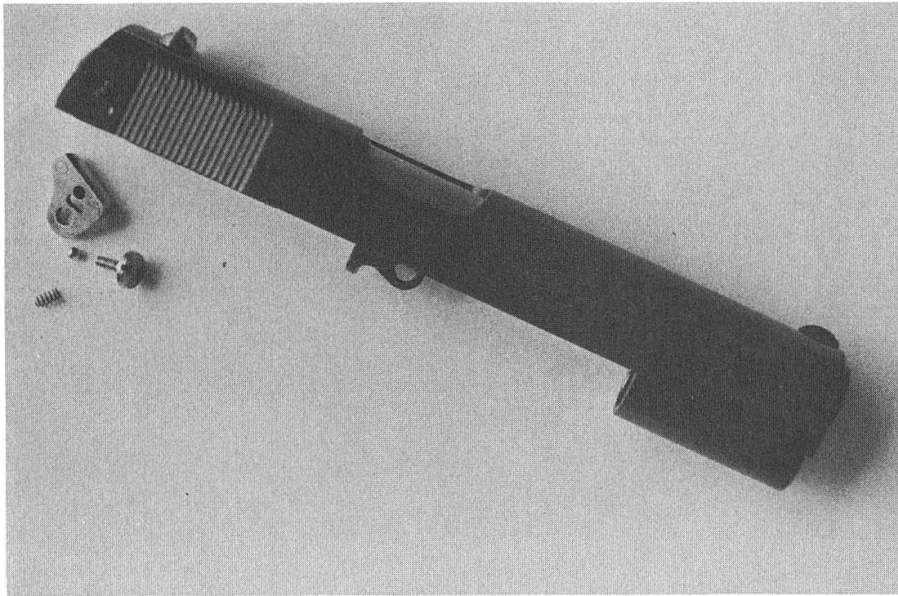
The lever type selector mechanism has been disassembled from the slide. The only visible modifications on this type of arrangement are four small holes. One hole is for the selector assembly screw that is threaded to take a standard 6-32 screw positioned at the end of slide. The center hole is for the stop pin, while the two shallow holes are for the selector index notches.
