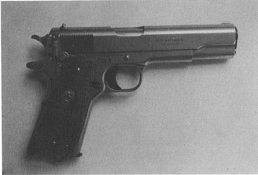
Right side view of the Colt .45, converted to a selective-fire configuration. The above Colt has the sliding type selector mechanism mounted on the vertically positioned dovetail groove in the rear portion of the slide. Note that the selector is set in the full auto position.
