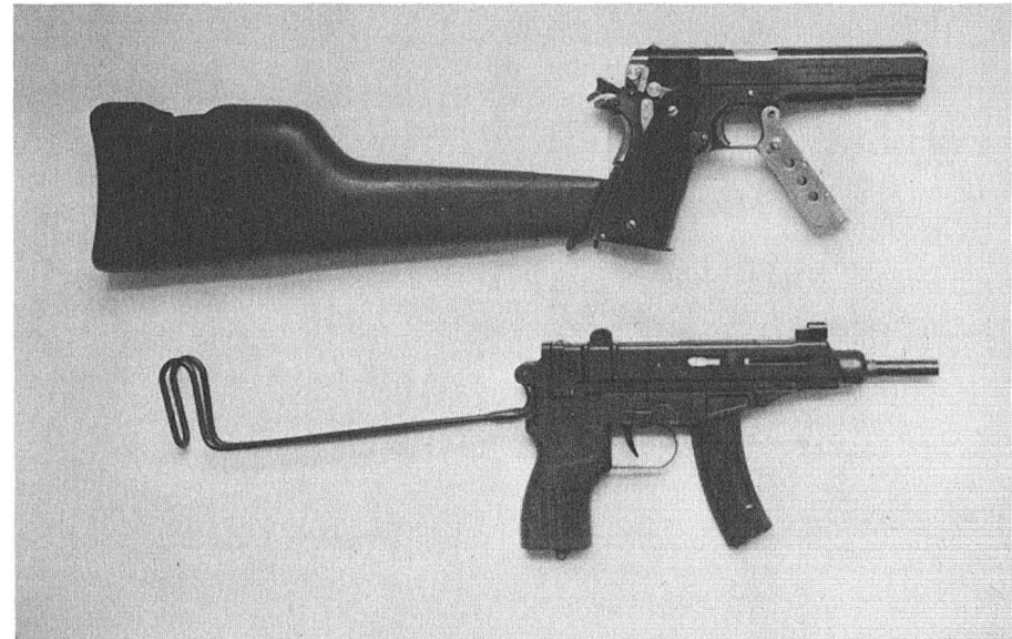
Same two guns with their stocks in the ready-to-use position. While the Colt .45 has the detachable Browning Hi-Power stock slid in, the Skorpion has its retractable wire stock extended. The Colt fires from the closed, locked breech system, while the Skorpion is an open-bolt "blowback" design, using a retarder mechanism to slow the rate of full auto fire.
