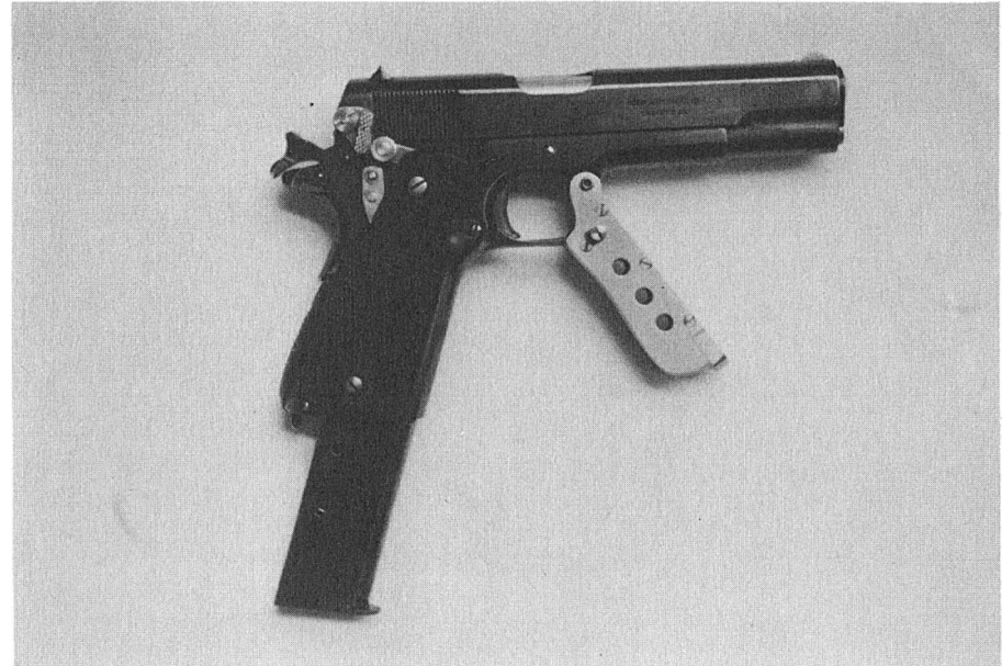
Right side view of the same gun with the hammer in the full-cocked position. The selector is set at full auto, and the front grip is shown in the retracted position. Note the long, straight magazine.
