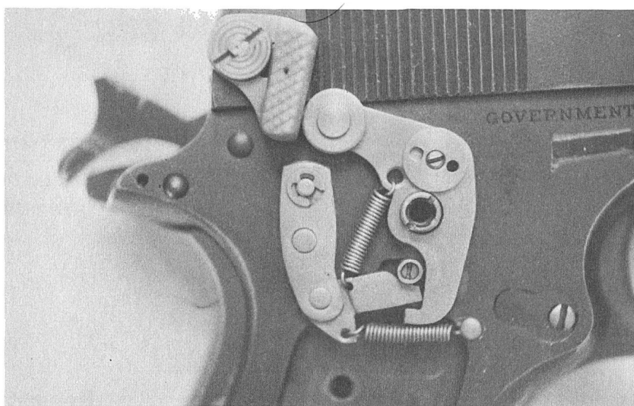
Closeup view of the Colt, with the other cam bushing substituted. Note the sear connector lever toe is resting over the tripper toe (lower portion of tripper) and against the cam bushing of the trigger bar. The connector always rests in this position as long as the trigger is not pulled (whether the selector is set on semi or full auto) to prevent accidental tripping of the hammer when the selector hits the roller during forward closing of the slide while in the process of loading (but not firing).
