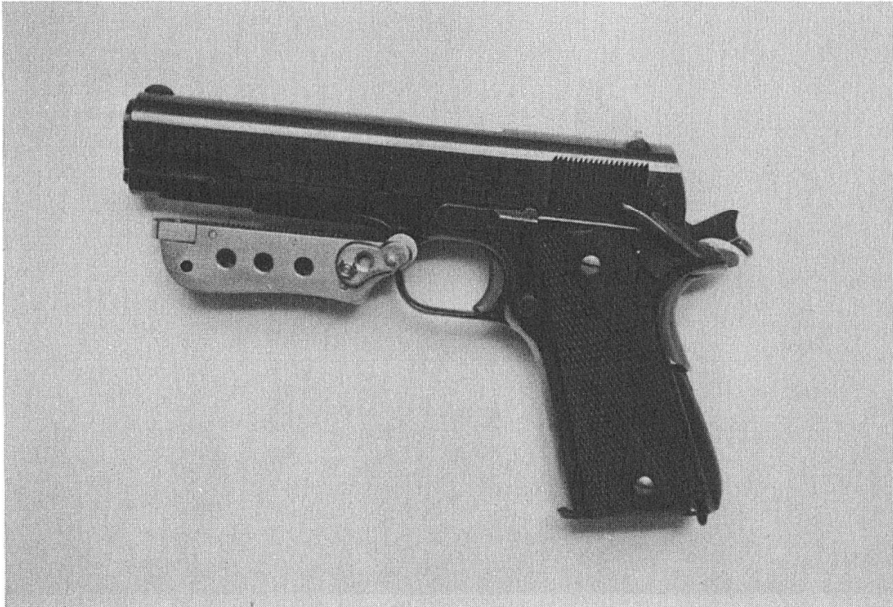
Same gun viewed from the left. The hammer is cocked, and the safety is on. The front grip is in the folded position. The locking piece containing the index on the top portion of the grip is operated by the push-button catch.
