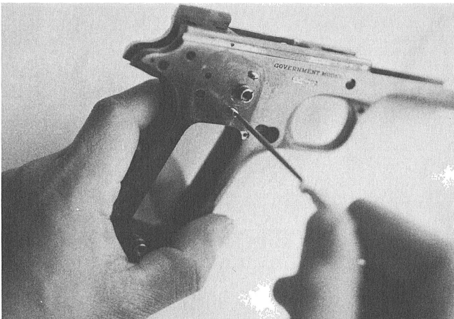
The cam screw protrudes past the slot and is fully tightened prior to the assembly of the converter mechanism. Both the trigger support screw and trigger bar cam bushing must be assembled before the converter unit is assembled to frame.
