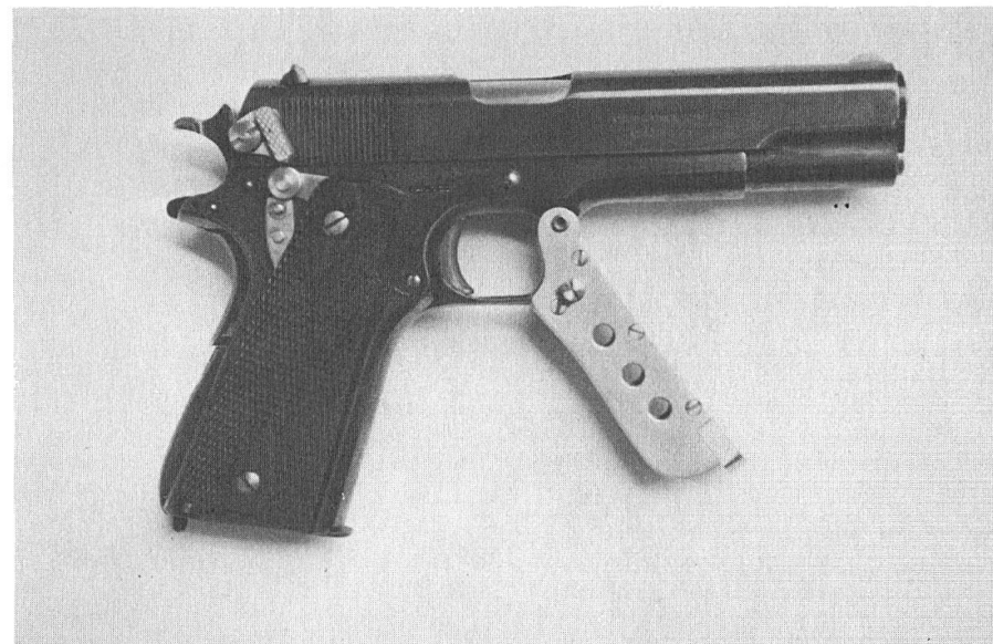
Same gun with the selector set at semiauto. The hammer is at the half-cocked notch. It is advisable to place the hammer in the half-cocked position before moving the selector from one index to the other. The slide needs to be retracted slightly (approximately 1/4 inch for the lever type selector and about 1/8 for the sliding type) to clear the roller so the lower end is not pressing hard against the tripper.
