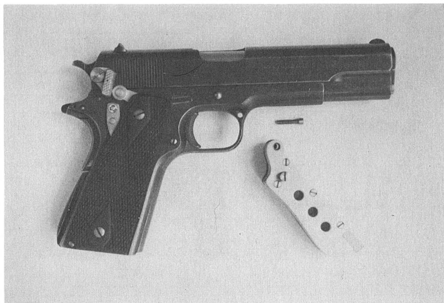
Right side view of another selective-fire arrangement, which has the lever type selector design. This gun operates the same converter unit mounted on the receiver frame that is used with the sliding type selector mechanism. The selector is seen in full auto position. The removable folding front grip is not assembled to the gun.
