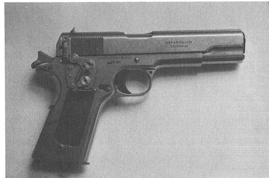
Same gun with the fire selector set at full auto, with the hammer in a cocked position.
