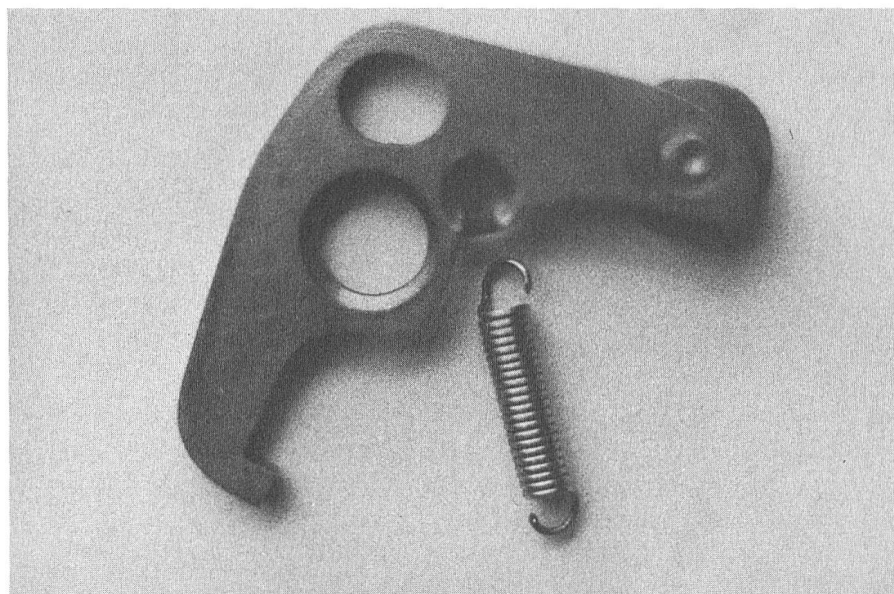
Same tripper turned upside down. Note the end of the roller rivet is flush to the surface of the tripper. The large center hole is assembled to the top grip screw bushing, and counterbored to accommodate the stop ring of the bushing in order for the tripper to lie flush on the receiver frame during assembly. The tripper spring is removed from its assembly hole.
