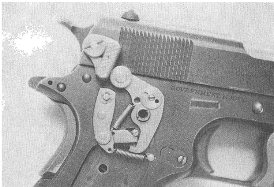
Proper relationship of converter mechanism with the hammer in the full-rest position and selector set at full auto. The trigger bar cam bushing is not assembled in place. The sear lever connector toe will rest slightly higher against the cam screw without the bushing in place.
