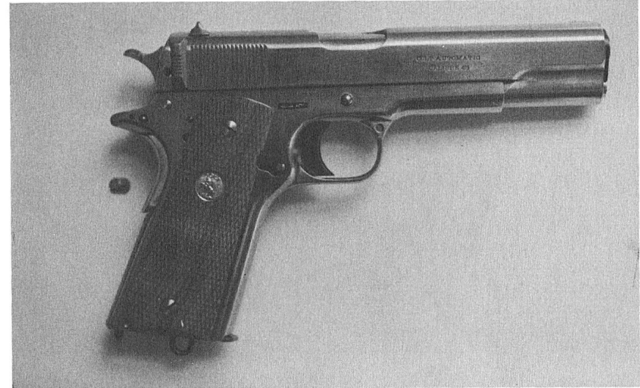
Same weapon with the selective-fire converter removed from the receiver frame. The fire selector was left on the slide. This gun will fire semiauto only, even when the selector is on. Note the small piece of metal behind the grip. This piece has a small, elongated lug which mates with the assembly slot of the sear lever trip pin. Half of this slot is partly visible below the sear pin hole. With this dropped in the slot, the slot will be covered completely. The thin wide portion is secured by the grip stock.
