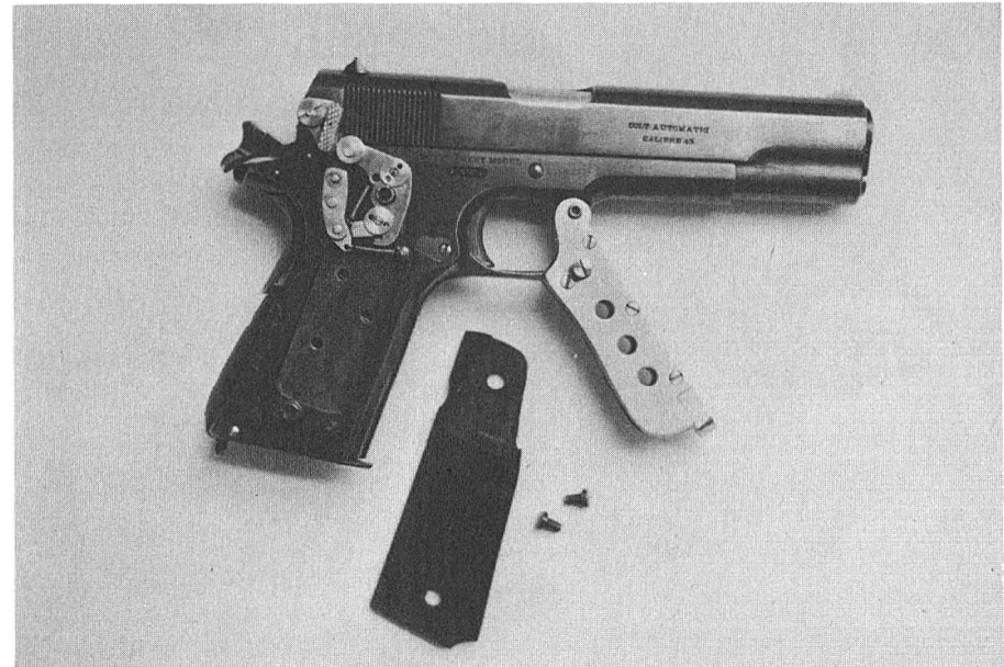
The right side stock is disassembled. The hammer is in the cocked position, the selector is set at full auto, and the front grip is in the retracted position.
