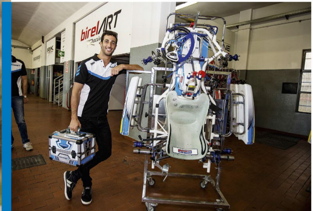
Ricciardo with the 125cc Birel ART kart that bears his name. Aimed at the serious young competitors Ricciardo is hoping to inspire, these karts produce over 40bhp and run in the KZ class
