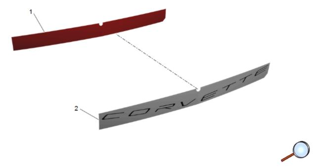
**Note:** When removing protective liners from the adhesive tape, be careful not to touch tape with hands and do not allow tape to come in contact with dirt or foreign matter prior to adhesion.
