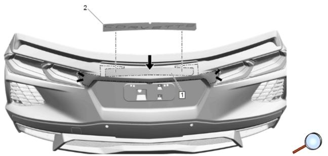
6. Position the emblem (2) with face liner and foam carrier to the rear bumper fascia (1) as instructed on template.
