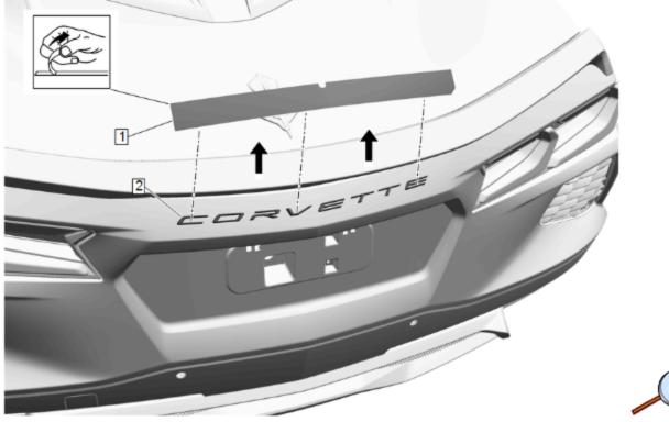
9. Carefully remove the face liner and foam carrier (1) from the emblem (2).
