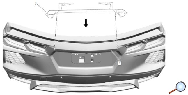
4. Position and tape supplied template (2) to the rear bumper fascia (1) as instructed on template.
