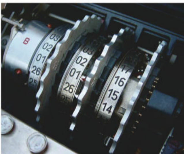
The three rotor stacks inside the Enigma machine were ingeniously replicated on the Bombe
