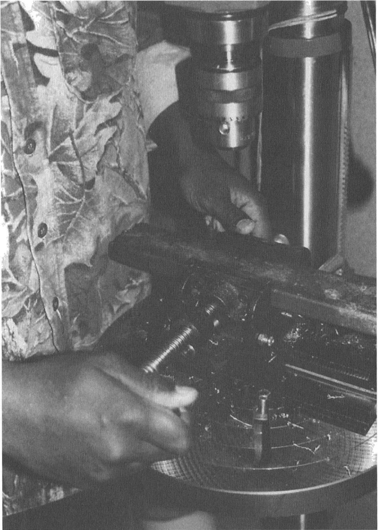
Setting up an adjustable drill press table to perform simple milling operations.
