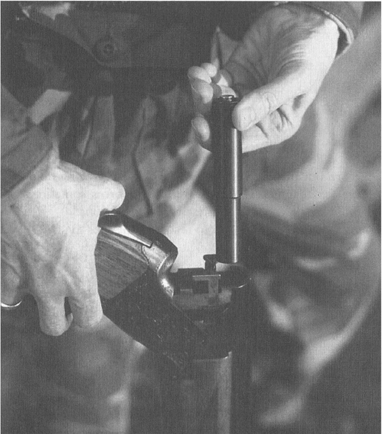
Inserting a 12-gauge adapter in a double shotgun.
