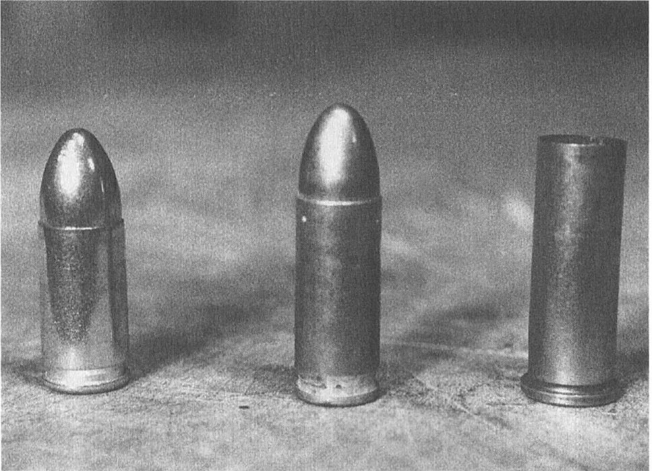
Left to right: factory 9x19; 9x23 made from .223 brass; .38 Special case which, with some work, can be made to work in a 9mm gun.
