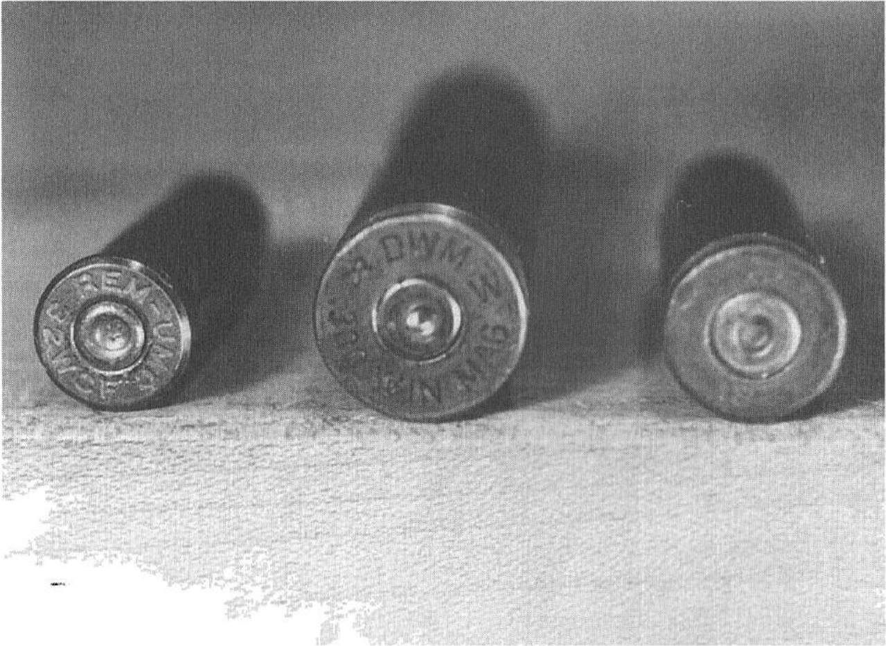
Reading pressures from primers. Left to right: rounded primer indicating low pressure; primer squashed flat against the firing pin and bolt indicating high pressures; primer from regular factory load.
