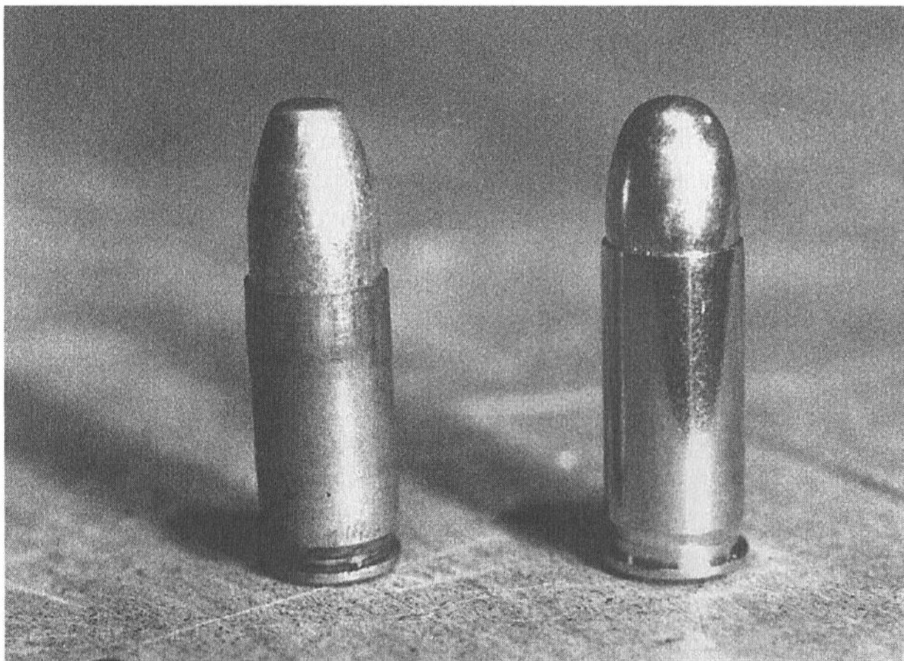
Factory 9mm Steyr (right) next to a 9mm made from .223 brass.
