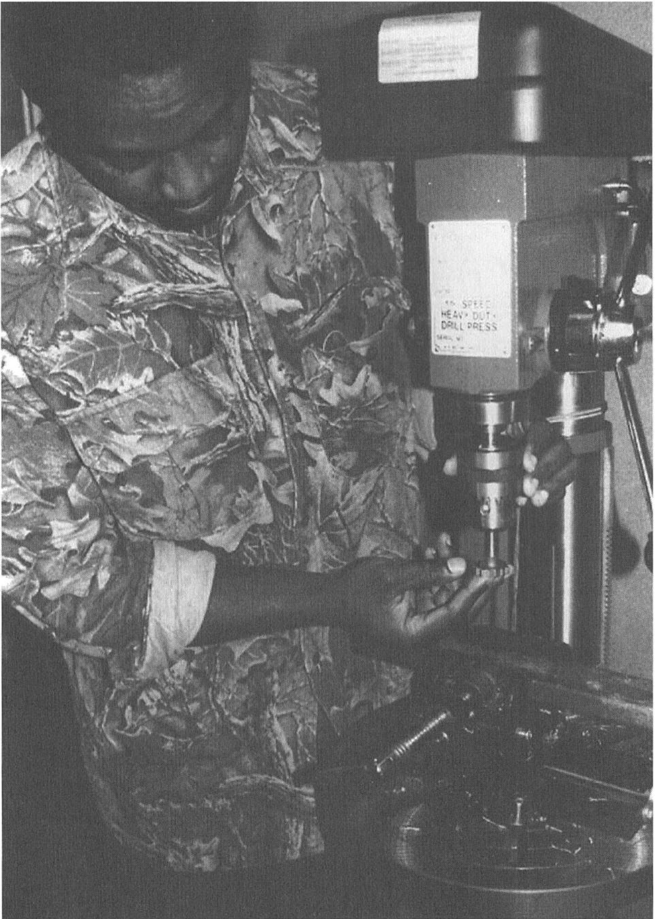
Inserting a common mill into a drill press in preparation for milling a piece of mild steel in the adjustable table.
