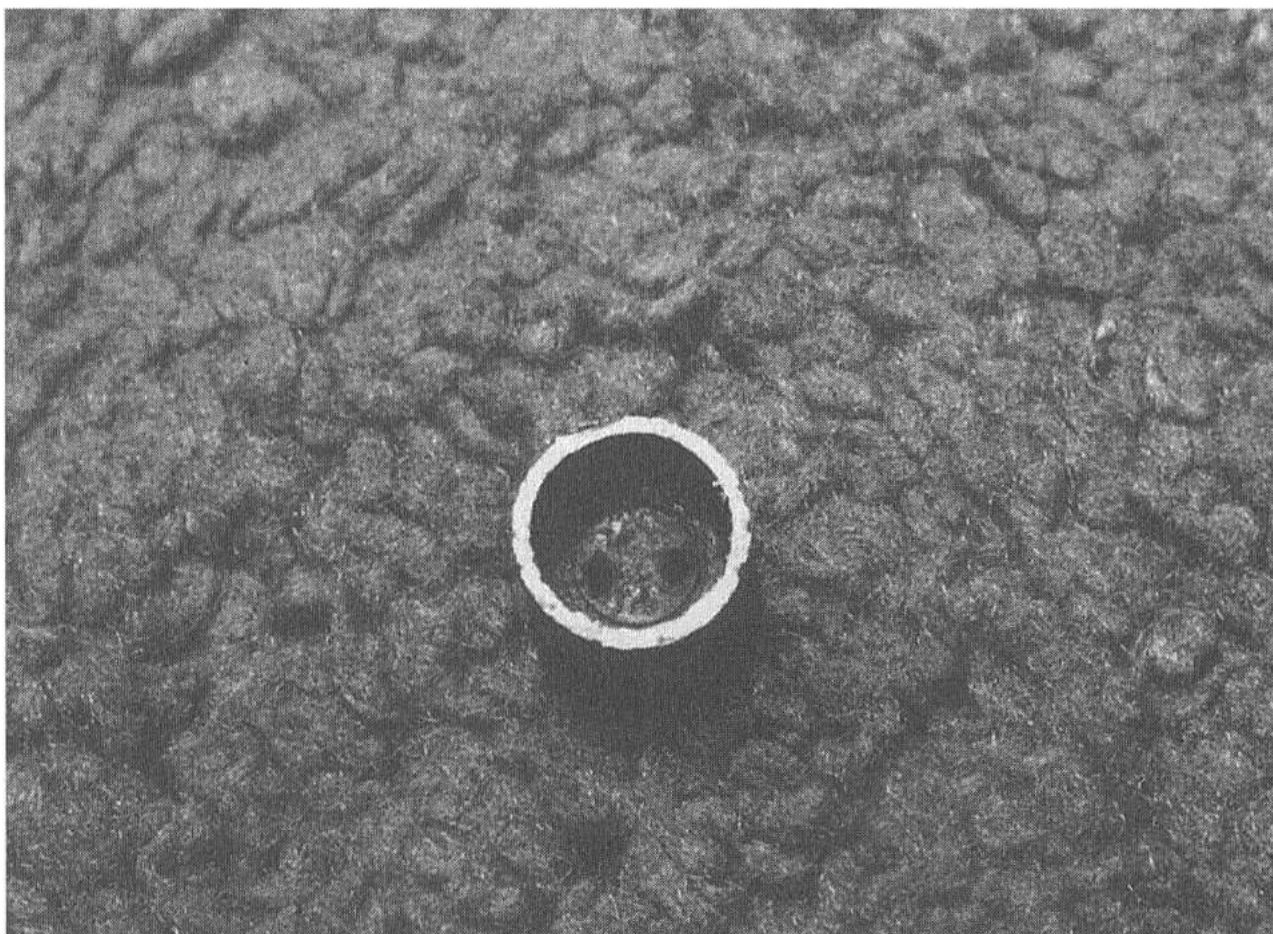
Berdan case cut down to show small flash holes that frustrate decapping by conventional means.
