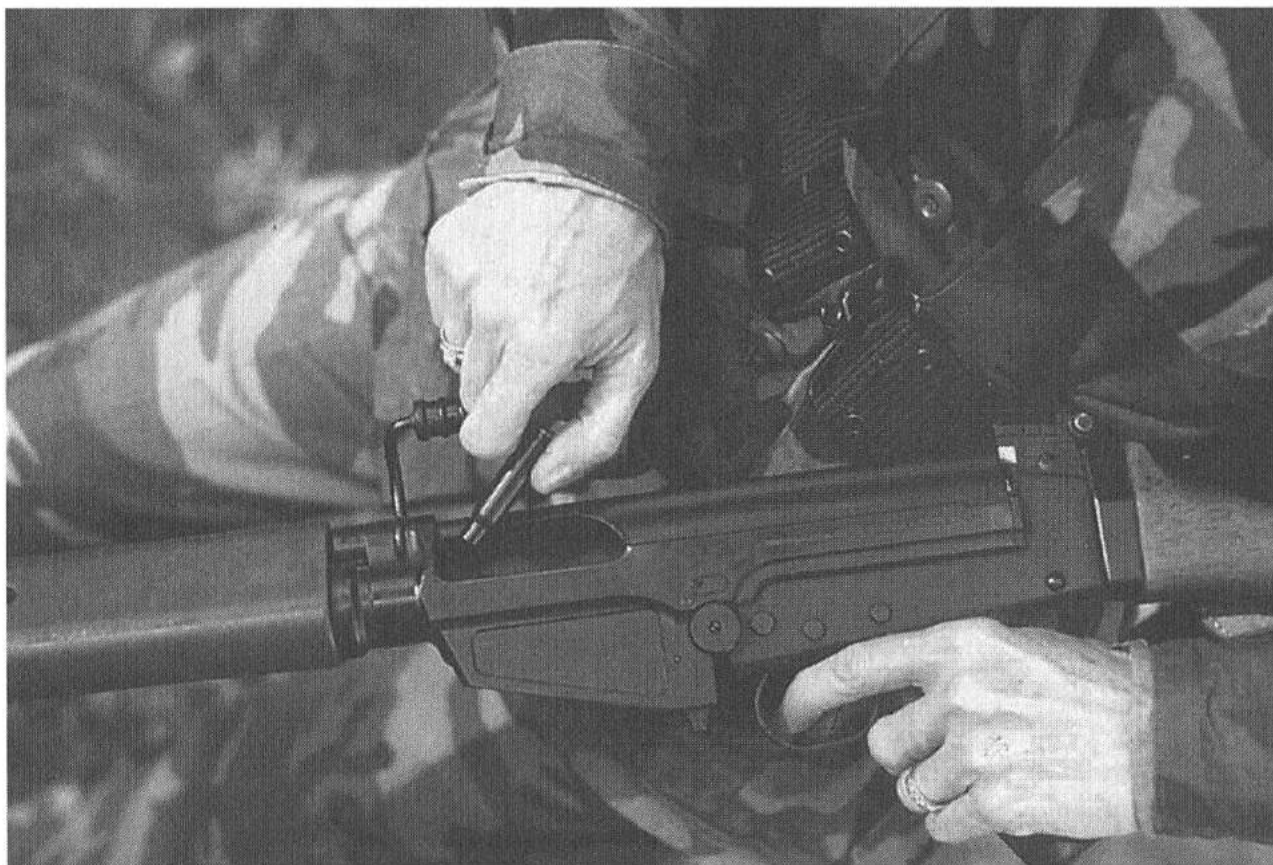
Inserting a loaded .308 adapter in an FN assault rifle.
